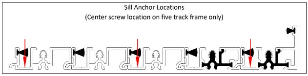
If the door has a spliced sill, mark holes on the splice plates.
