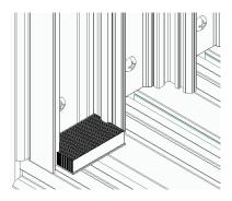
3.H. Sill channel foam plugs – With the panels closed, mark each interlock location at the sill on the interior and exterior. Move panels and insert a sill channel foam plug into the sill channel at each marked location. Plug will extend approximately 1/4" past the interlock in both directions. Ensure the plug is flush with the top of the sill.
