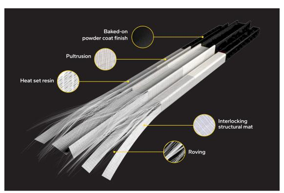
PROPRIETARY FIBERGLASS MATERIAL Pella's fiberglass windows and patio doors are made from our proprietary fiberglass material through our one-of-a-kind manufacturing process.
