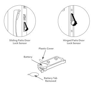
the plastic cover to expose the battery. Remove the plastic tab separating the battery from the device.
