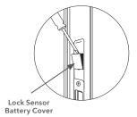
Replace battery cover on LOCK SENSOR. NOTE: Once the plastic tab is removed from the battery, you will have 2 minutes to pair your LOCK SENSOR to BRIDGE. If 2 minutes pass without successfully pairing, remove and insert the battery again. You are ready to pair LOCK SENSOR to BRIDGE.
