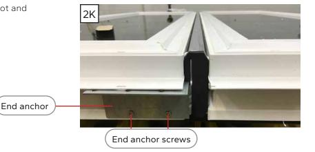
L. Fill the void with sealant from the fin flush to the exterior edge of the frame and insert the splice key as shown.
