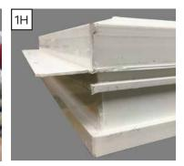
I. HORIZONTAL MULLIONS ONLY: Drill three 3/16" diameter weep holes through the first outer vinyl layer of the frame on the top (head) of the bottom unit in the location shown. One 6" from each end and one in the center. Off set the center hole if mulling composite units.
