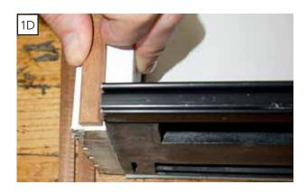
E. Use the provided template to position the molded nose correctly with the arrows pointed toward the door panel. Near one end, insert a staple next to the template.
