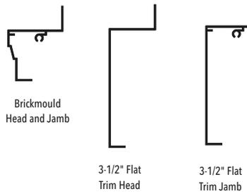
Brickmould Head and Jamb
