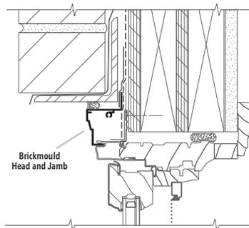
Brickmould Head and Jamb
