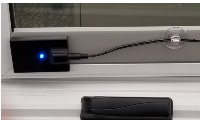
Inductive transmitter paired with receiver located on casement unit, with wire facing interior. If needed the suction cup included can help keep some of the cord weight off of the charger.
