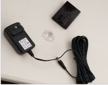
Shown is the 12V wall adapter cord, Inductive Charger Transmitter, and suction cup, all included in the charging kit.
