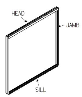
b. Ensure the end plates on both ends of the Head and Sill (if applicable) are secured.
