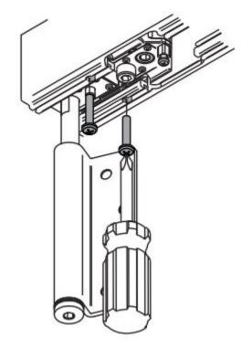
f. Once the top pivot is installed, loosen the locking screw and turn the adjustment screw such that the top hinge is touching the surface of the jamb. (See *Brio* adjustment instructions for details).
