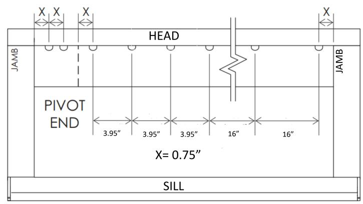
6. Use recommended anchors (#10 -  $3 \frac{1}{2}$ ") to secure the head to the header
