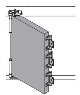
b. Hold the next panel in the sequence and attach the panel using the predrilled holes and provided anchors.
