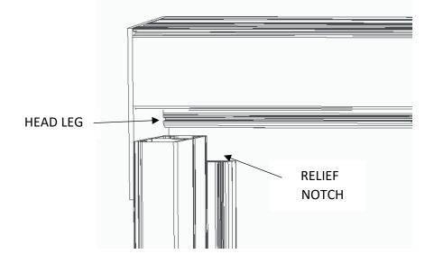
3. Justify the end of the jamb to the bottom surface of the head and the back of the jamb to the endplate.
