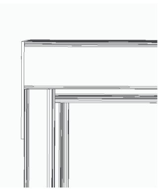
4. Locate holes in the jamb and confirm alignment with the through holes on the endplate.
