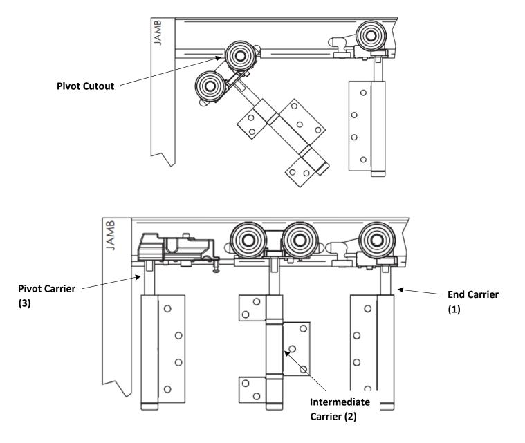
e. After the insertions of hardware into the slot, anchor the Pivot carrier through the two pilot holes in the head.
