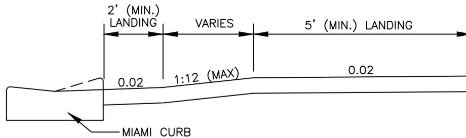
**SECTION THROUGH RAMP RUN AND LANDING**
