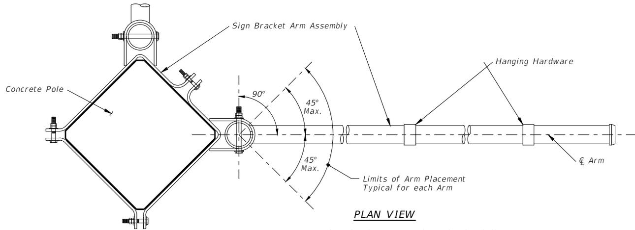
Concrete Strain Pole Shown - Round Steel Pole Similar
