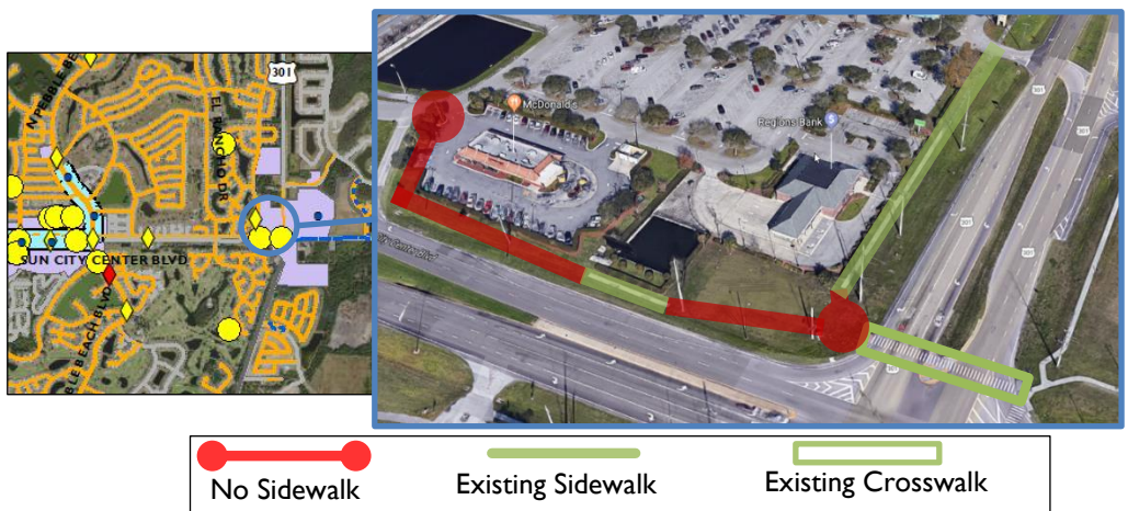
Figure 44. Pedestrian network at US 301 and Sun City Center Blvd.
