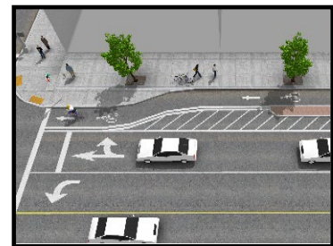
Bicycle Approach to an Intersection, Source: NACTO
