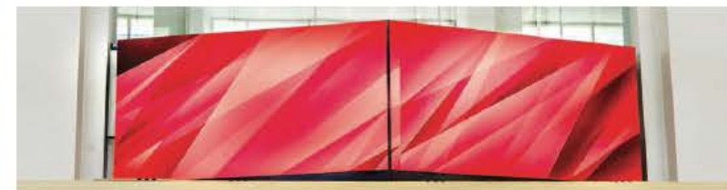
Hall A Video Marquee Video Wall Full Screen: 1920 (w) x 512 (h) Split Screen: 960 (w) x 512 (h)
