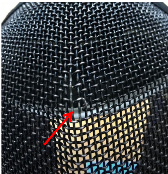
Examples of broken or damaged wires in the mask mesh
