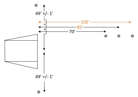
h. Along with the 70 ft., 85ft., and 100ft. distance buoys, there shall be corresponding 70 foot, 85 foot, and 100 foot markers on shore. These markers will be used to form a line with their corresponding water buoy in order to ensure a consistent measurement.
