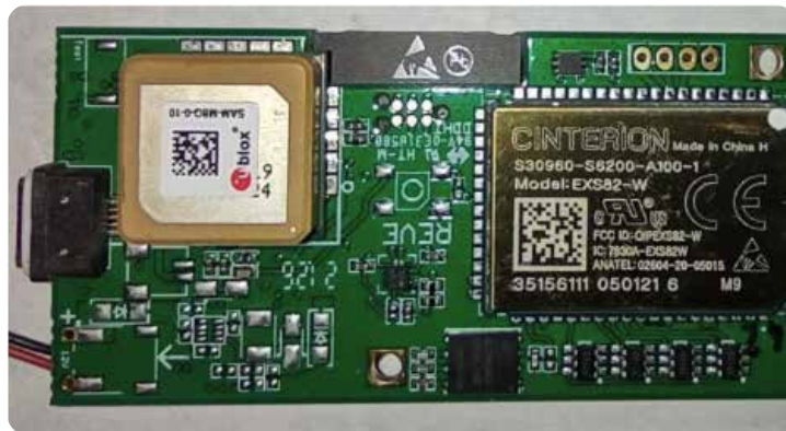
Figure 4. Cinterion Cellular Module in GPS Tracker
