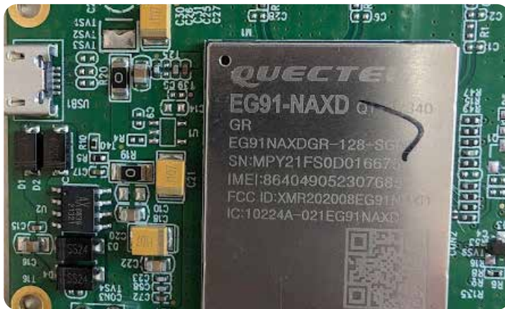
Figure 1. Quectel EG91-NAXD on Field Camera PCB
