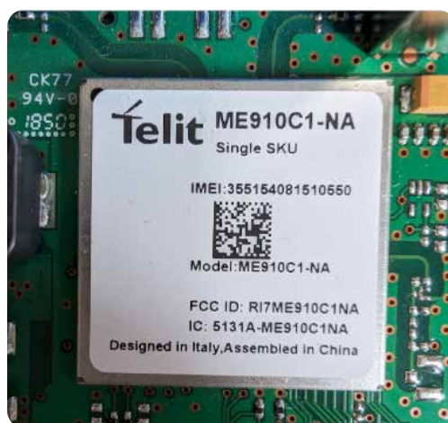
Figure 3. Telit ME910C1-NA in Cellular Modem
