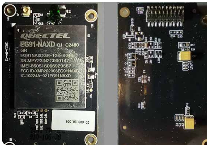
Figure 21: Quetecel EG91-NAXD on Trail Camera's PCB
