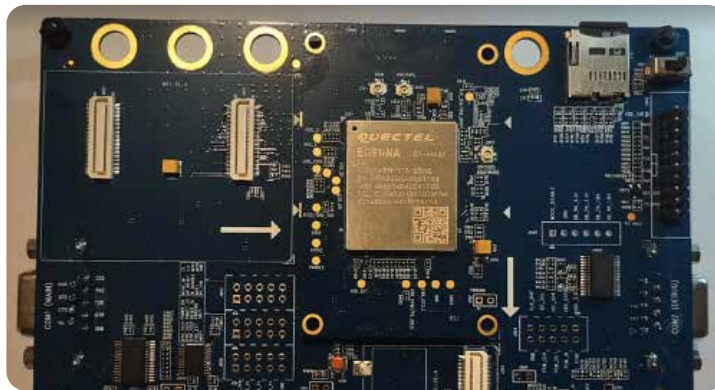
Figure 11. Quectel UMTS&LTE-EVB-KIT with an EG91-NA module
