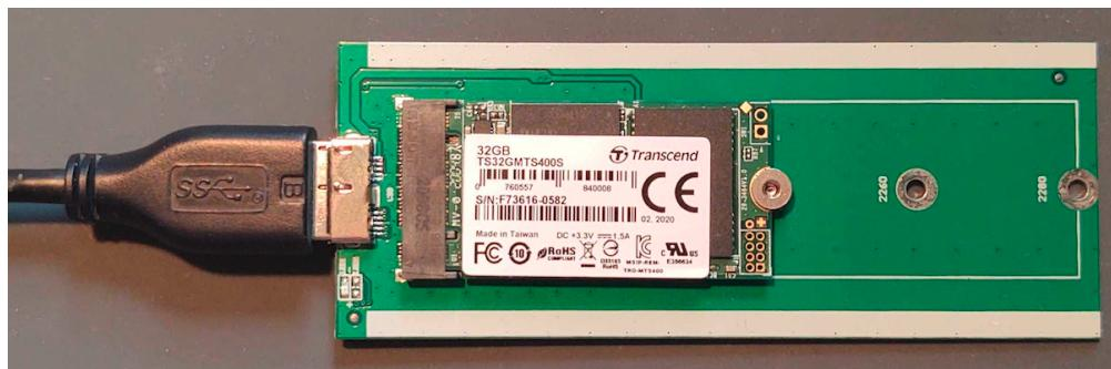
Using the SSD mounted in the USB reader, we examined the device for
