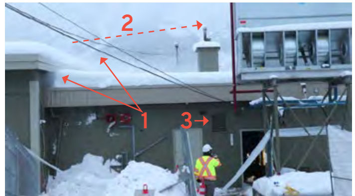
Photo 14 (above): Smoke test showing roof above mechanical room. Smoke became trapped (1) in depression between curling and arena roofs and was observed moving toward the roof edge rather than up into outside airstream (2). The air inlet for the furnace room for the building is identified (3).
