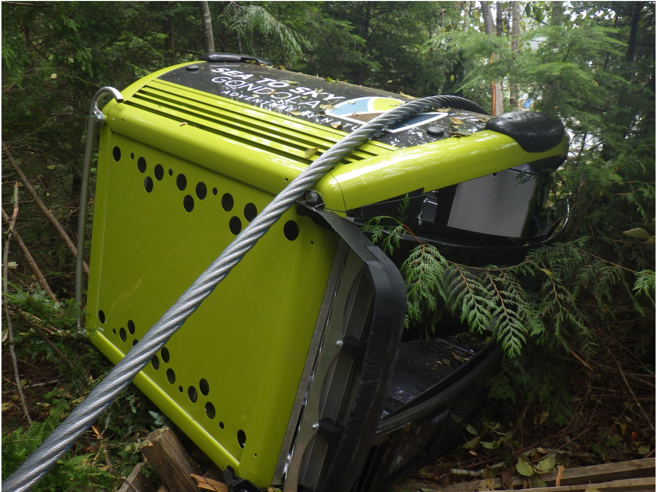
Image 4 – Damaged gondola cabin in the woods with the haul rope laying on top
