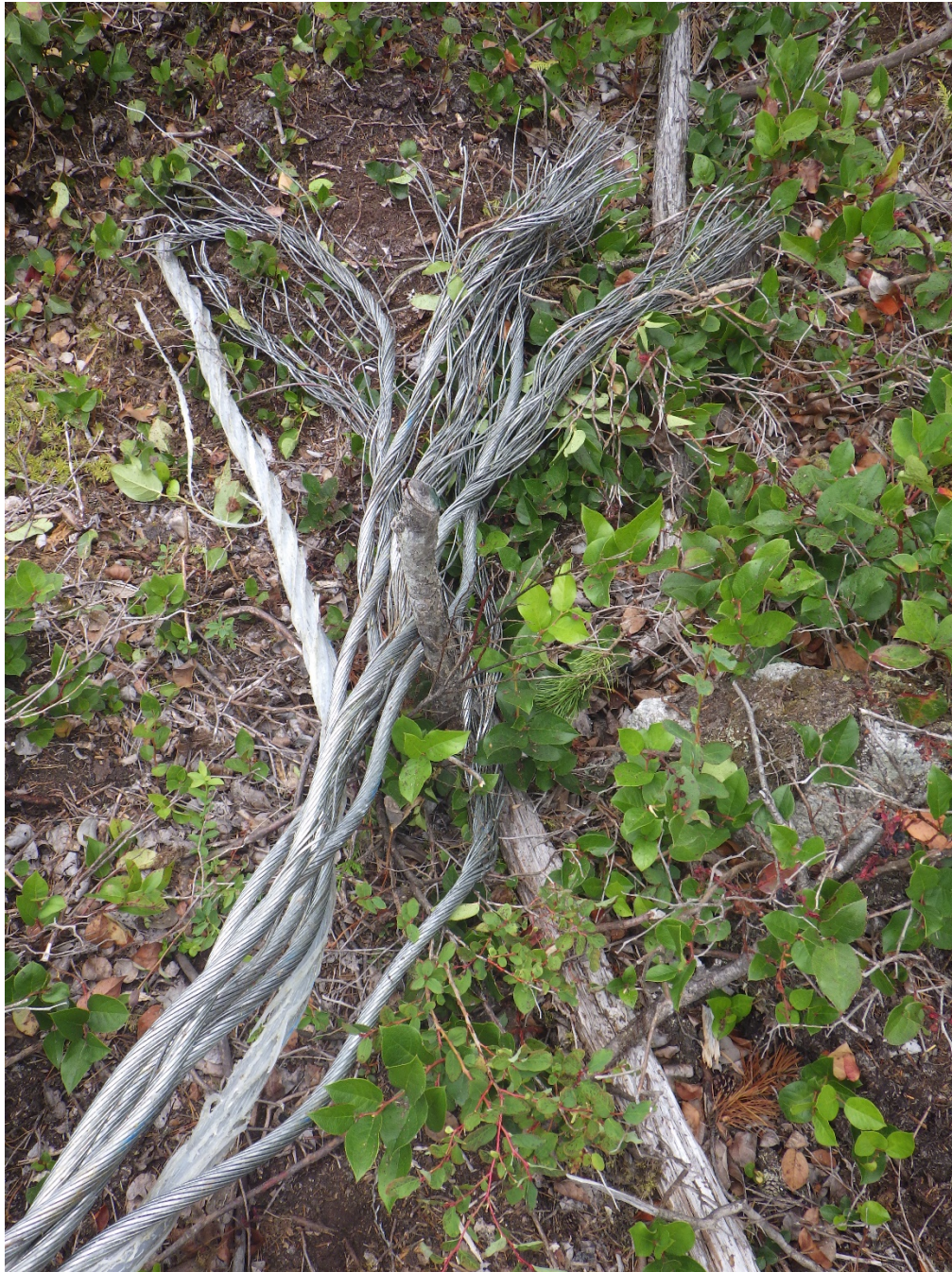
Image 8- Upper end of cut haul rope showing strands, wires and plastic core
