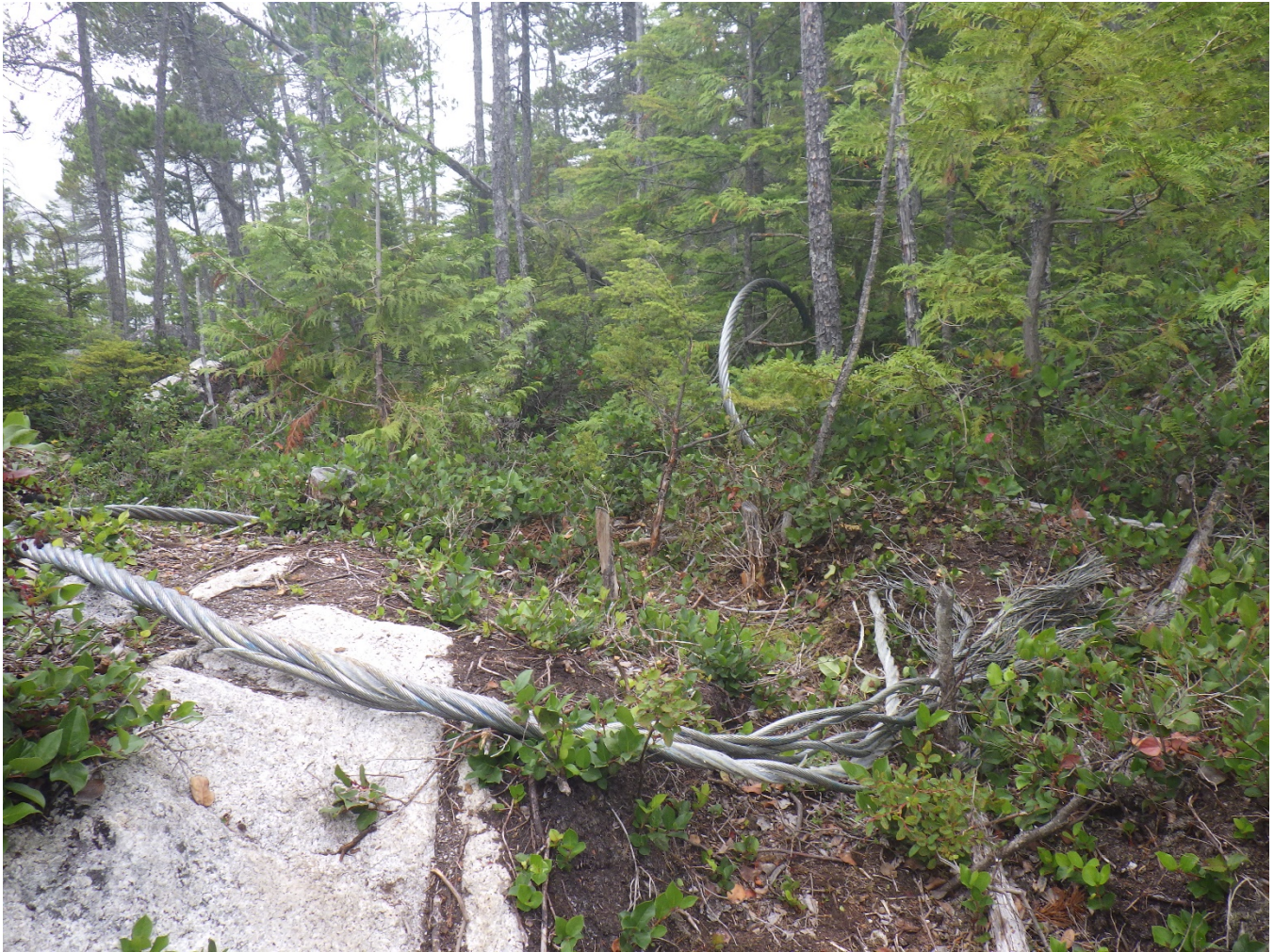
Image 7 – Upper end of cut haul rope as found
