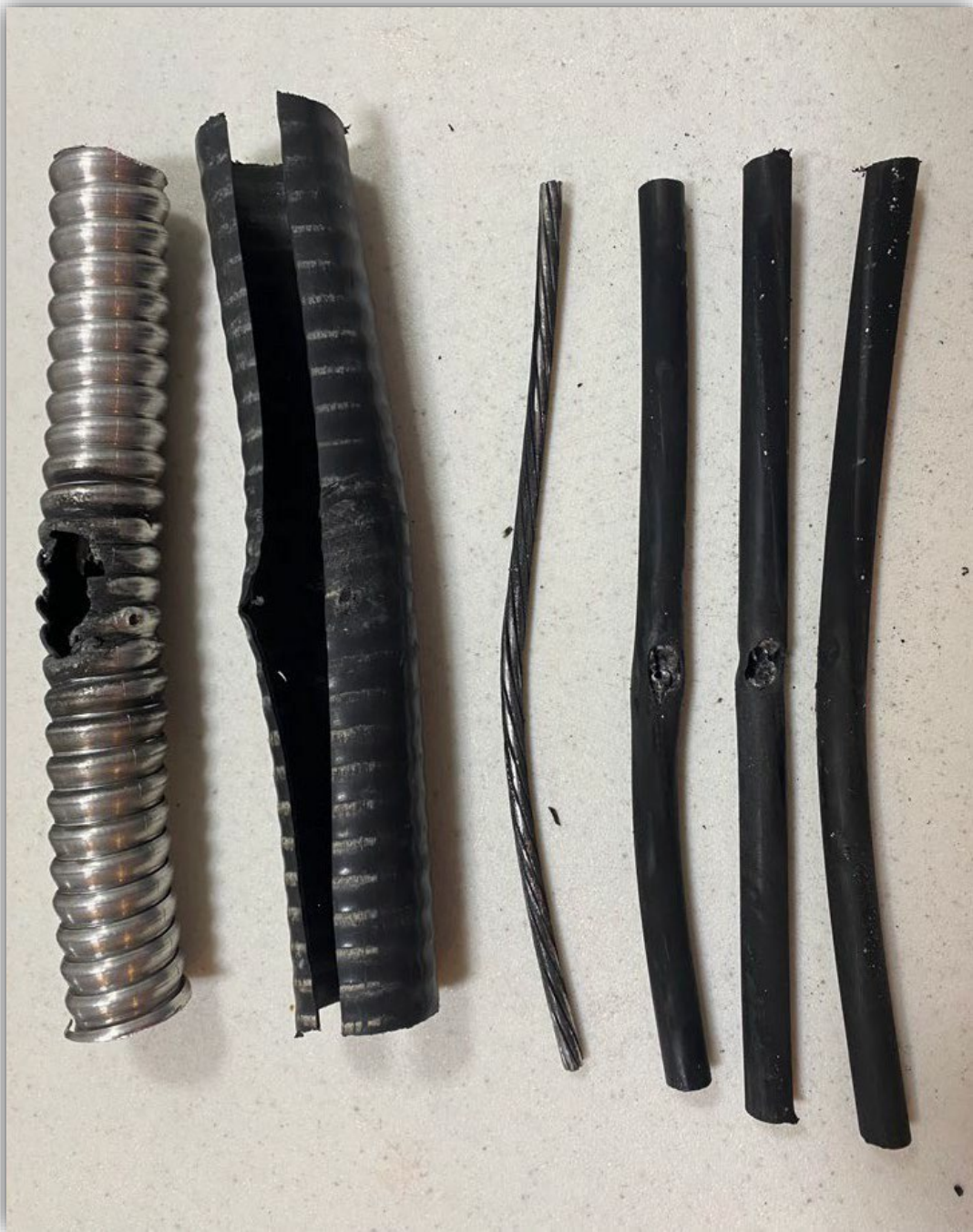
Image 3 - All components of the 300mm section of damaged ACWU cable.
