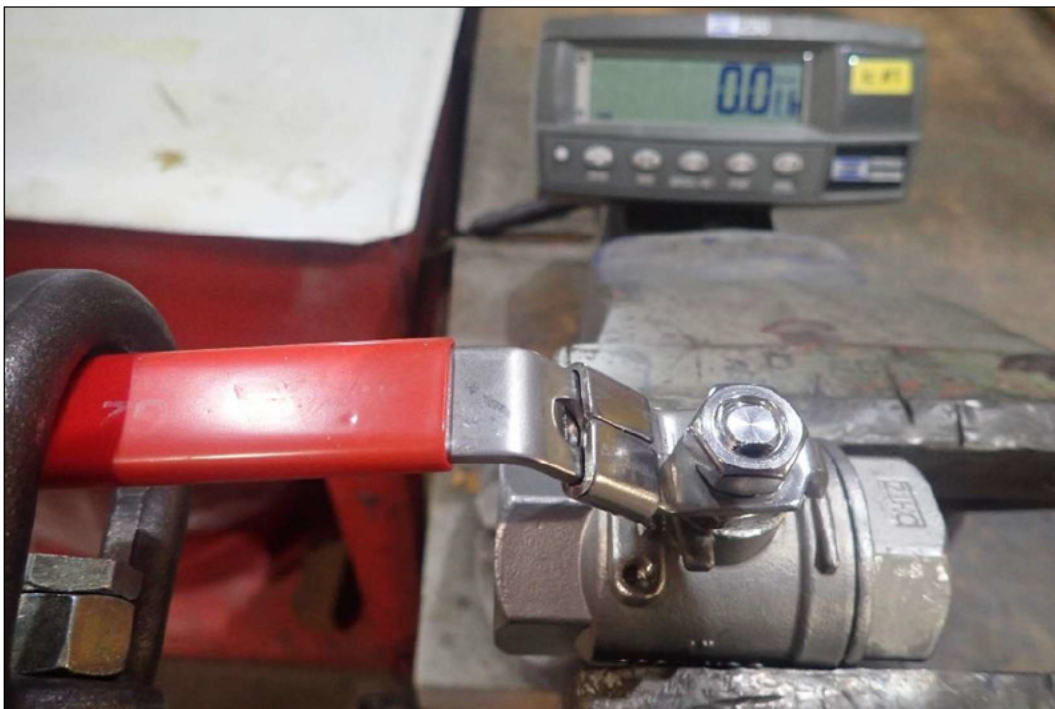
Figure 11 Load measuring system used for determining operating loads on valve.
