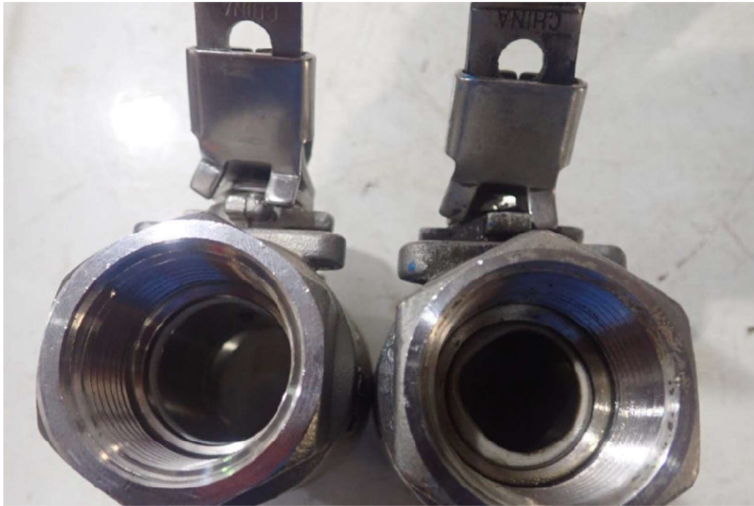
Figure 17 Simulated overload of locking device on #2 valve (left side). Subject #1 valve shown on right for comparison.
