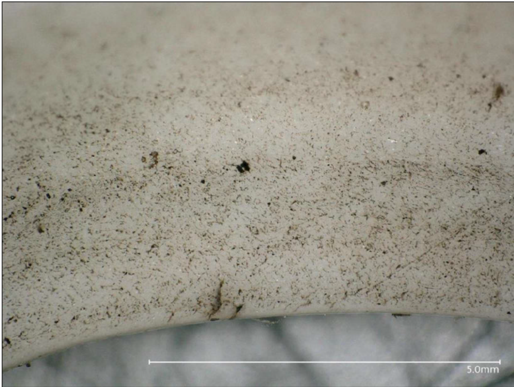
Figure 16 Close-up view tear shown at arrow in Figure 15.
