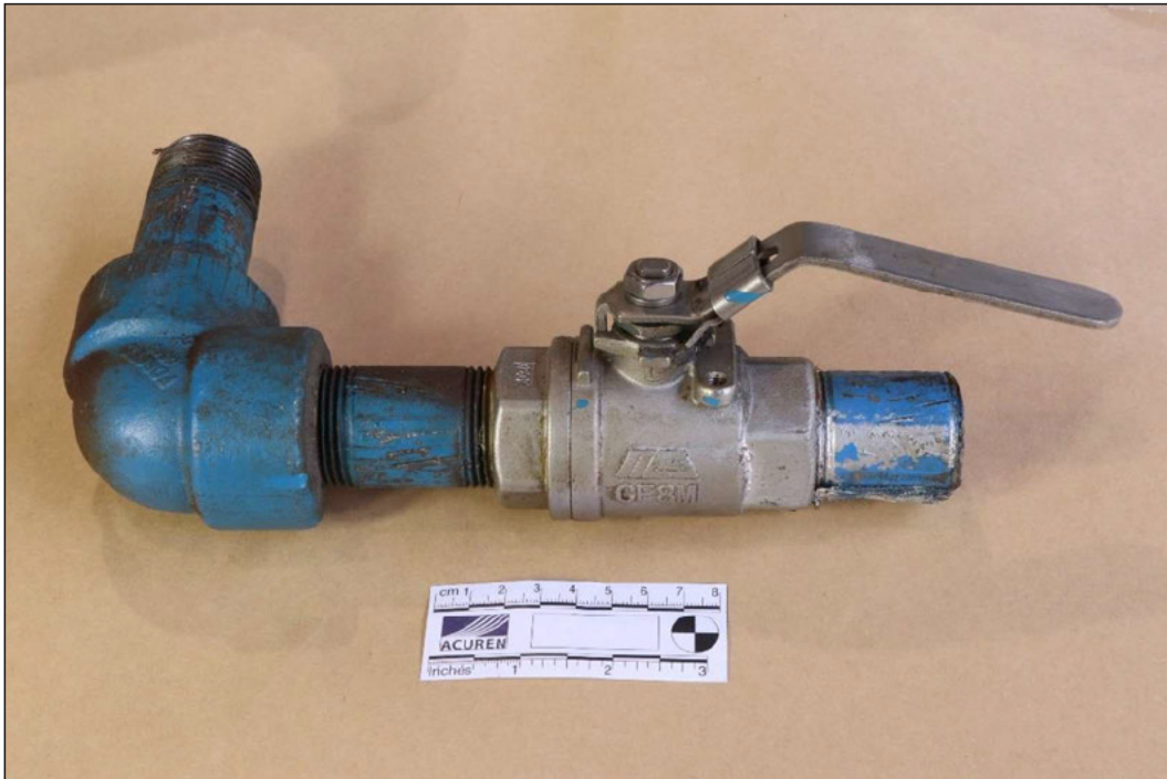
Figure 2 Overall view of subject valve with attached fittings and pipe segment. Valve was mounted vertically with pipe segment in the "up" position.
