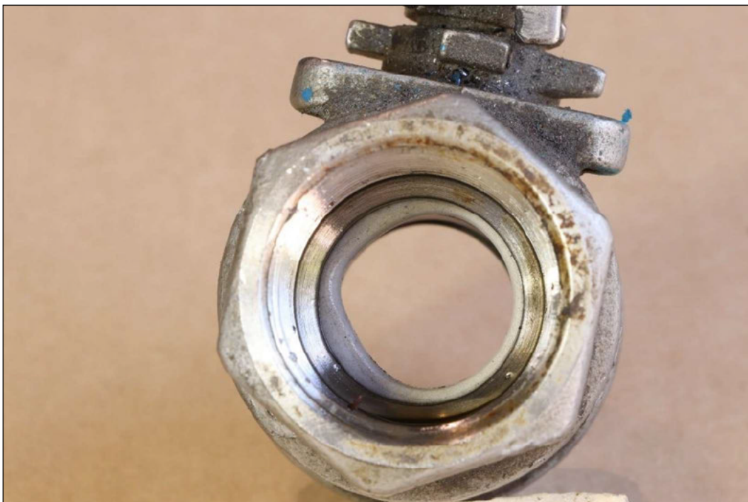
Figure 9 Deformation in outlet seal partially blocking 1" diameter hole.
