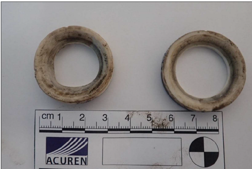
Figure 13 Seals removed from subject valve. Deformed outlet valve is on left.
