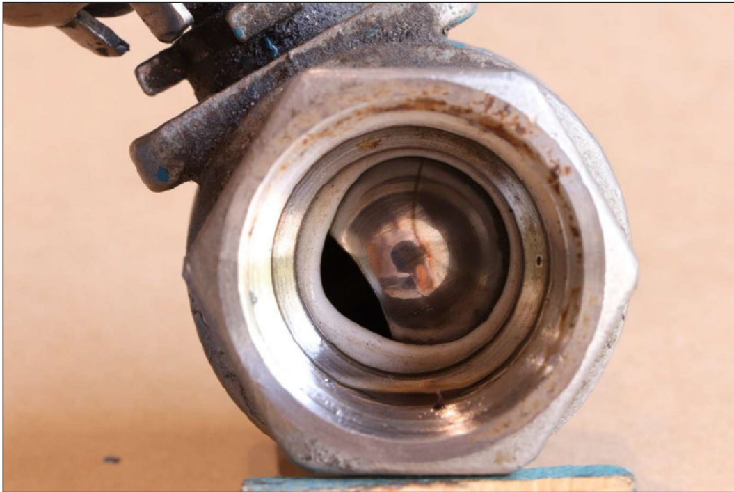
Figure 14 Valve opening at 45° lever movement. Note maximum seal deformation is at location of partial opening.
