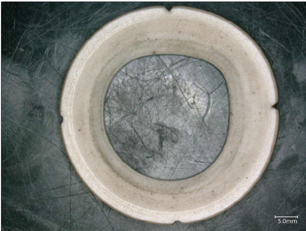
Figure 15 Close-up view of cleaned outlet seal. Most severe deformation is at upper right. Small tear is at arrow.
