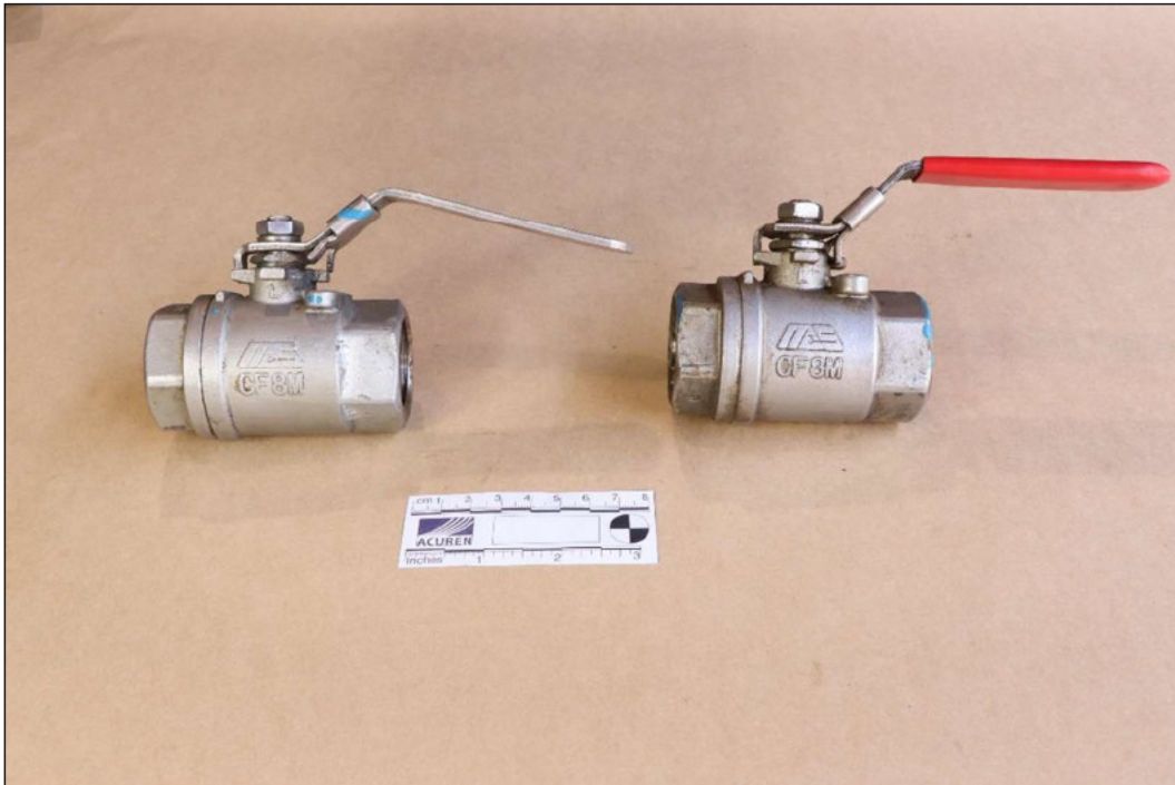
Figure 8 Subject Valve #1 and Valve #2 side by side showing permanent bend in Valve #1 lever.
