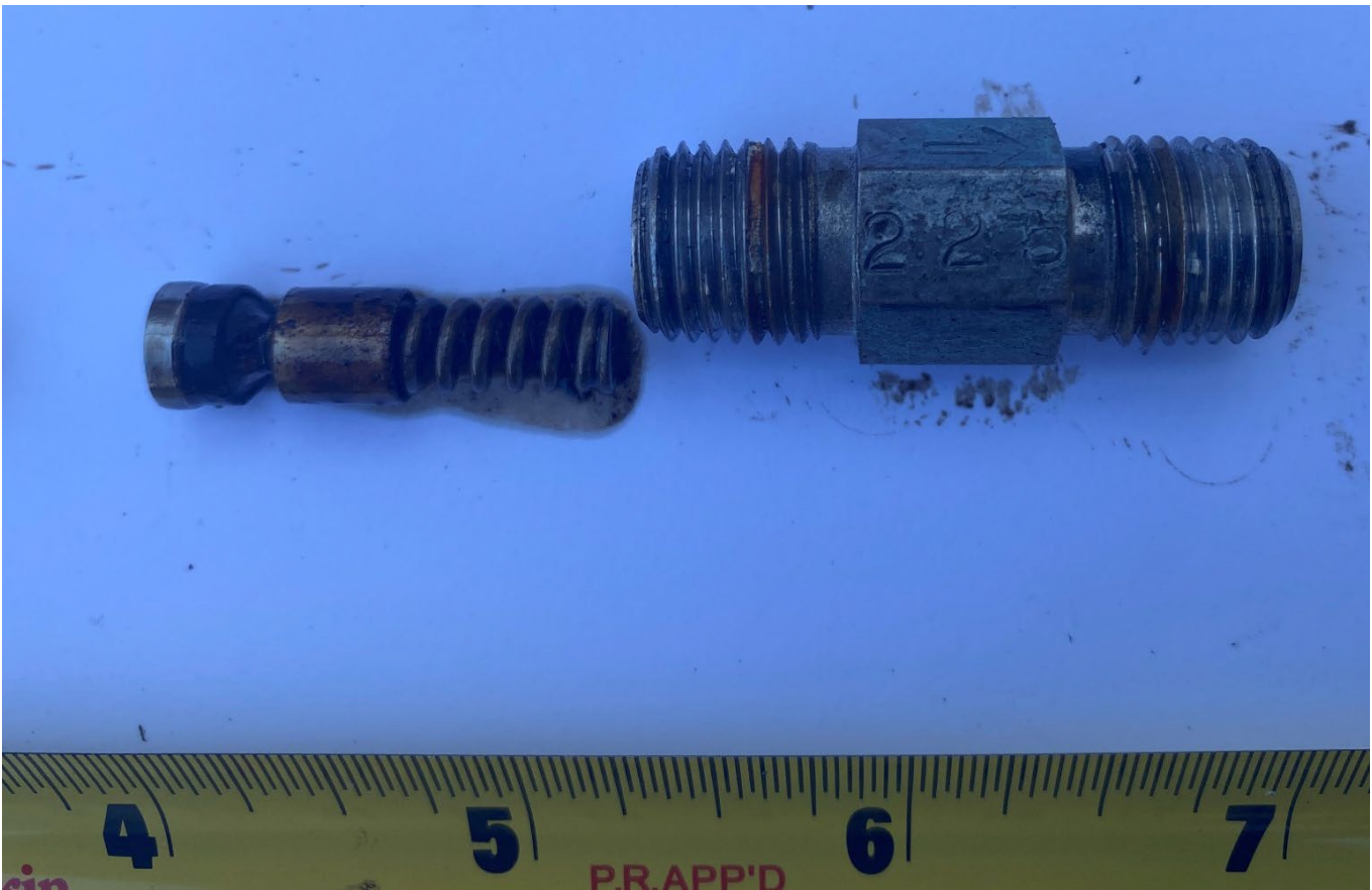
Image 9 – The auto-purger relief check valve showing oil saturation of the internal components.
