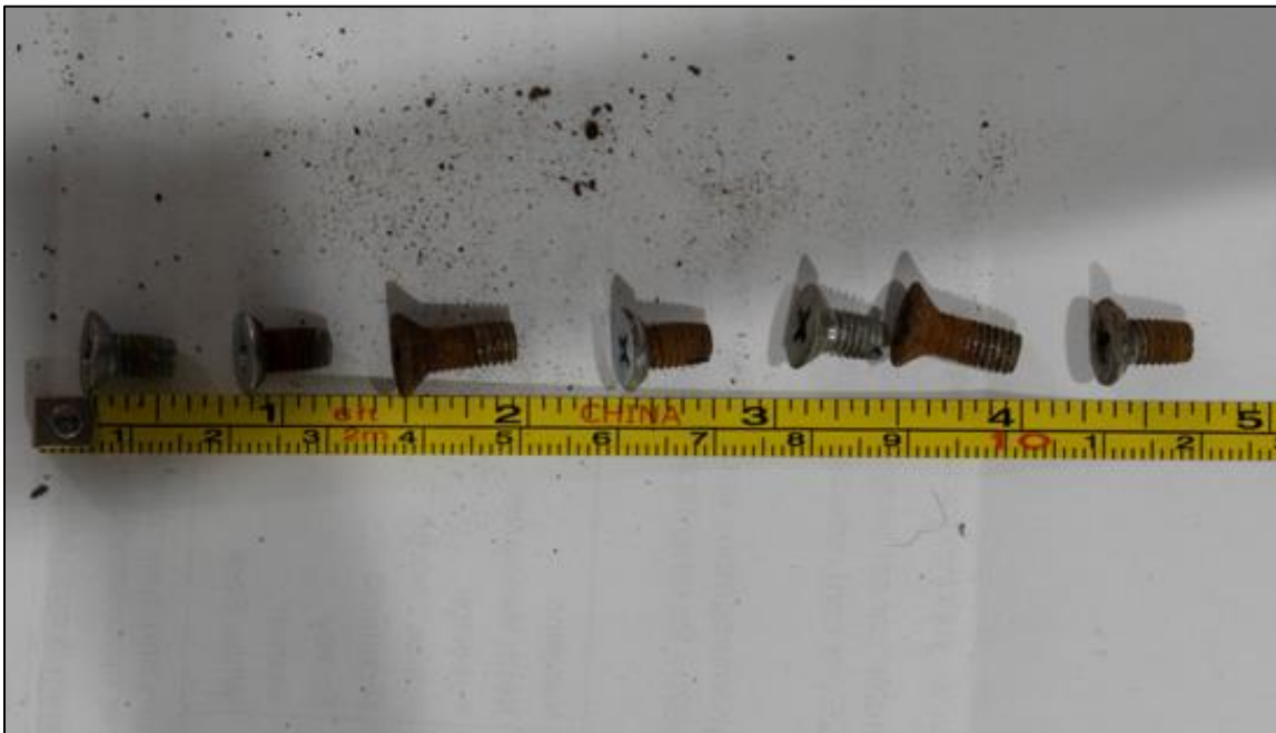
Photo 4: Door gib mounting screws – exposed threads show corrosion
