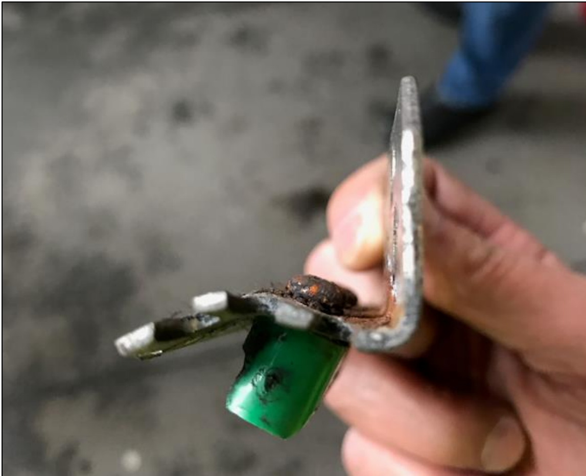
Photo 3: Door Gib - Devices on bottom of sliding door panels which fit into sill grooves and hold the door panels in alignment.
