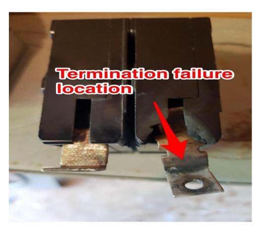
2 Pole 90 Amp breaker shows overheating on one side only
