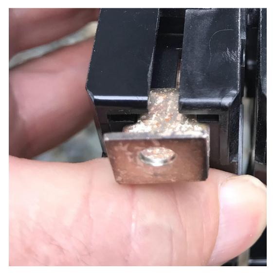
Termination point on the side of the breaker that did not fail. No arcing, pitting or signs of overheating.
