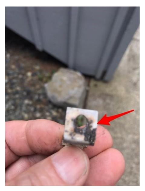
Arcing and pitting on the back of the termination pad
