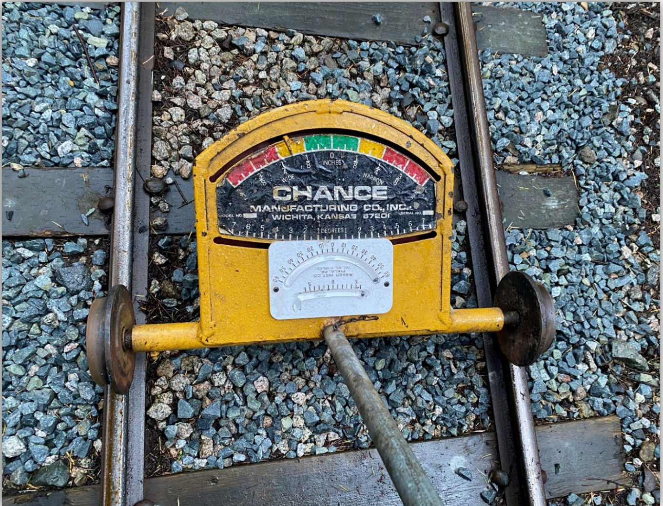
Image 6 – Chance track gauge in use after it was repaired after the incident.
