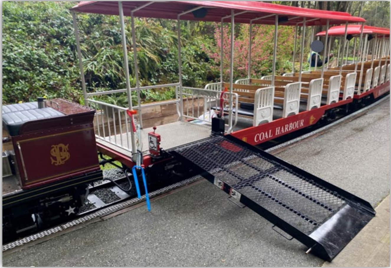
Image 3 – Accessibility ramp unfolded at the loading station.
