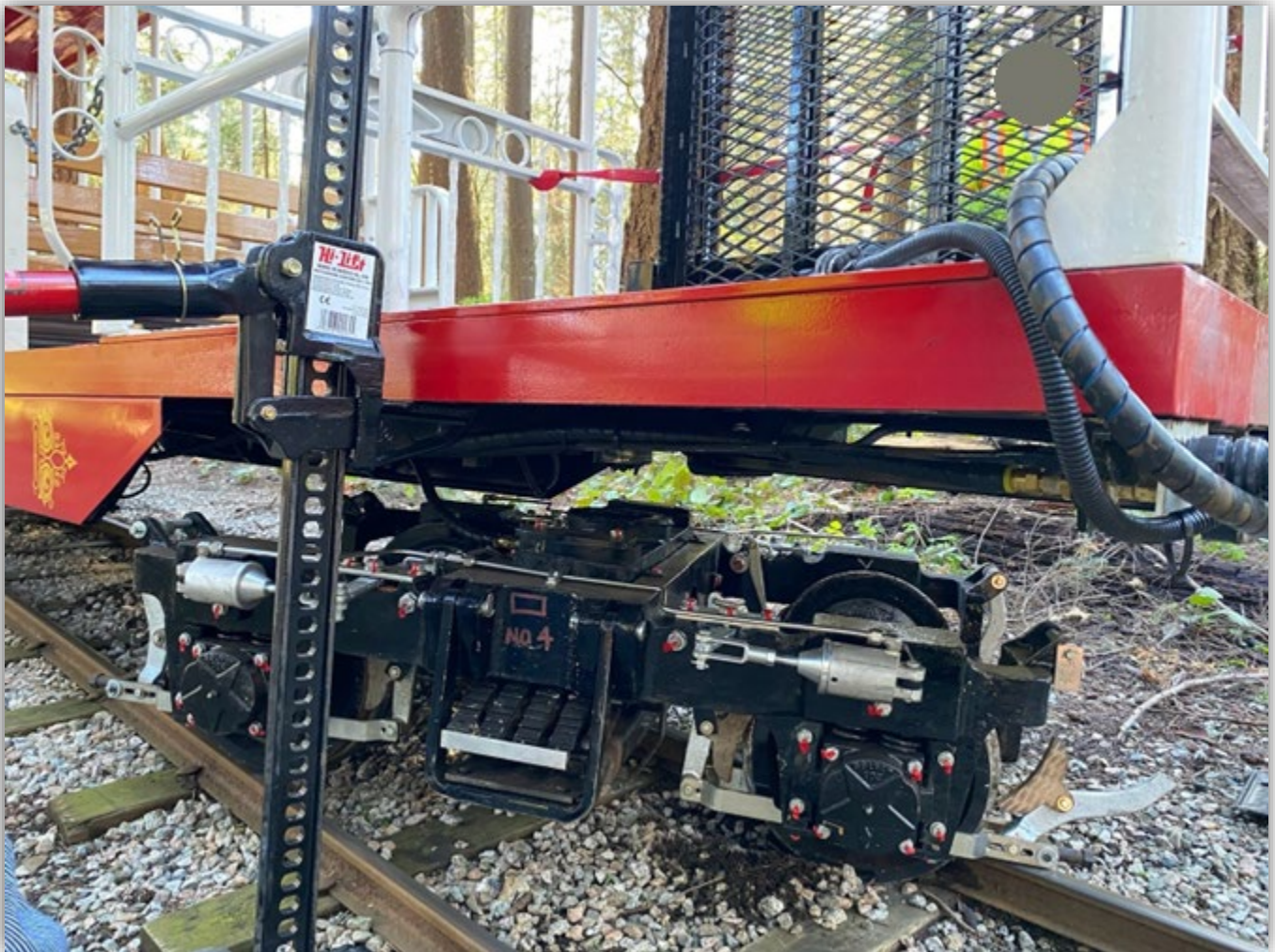
Image 1 – The accessibility car jacked up and the derailed bogey.
