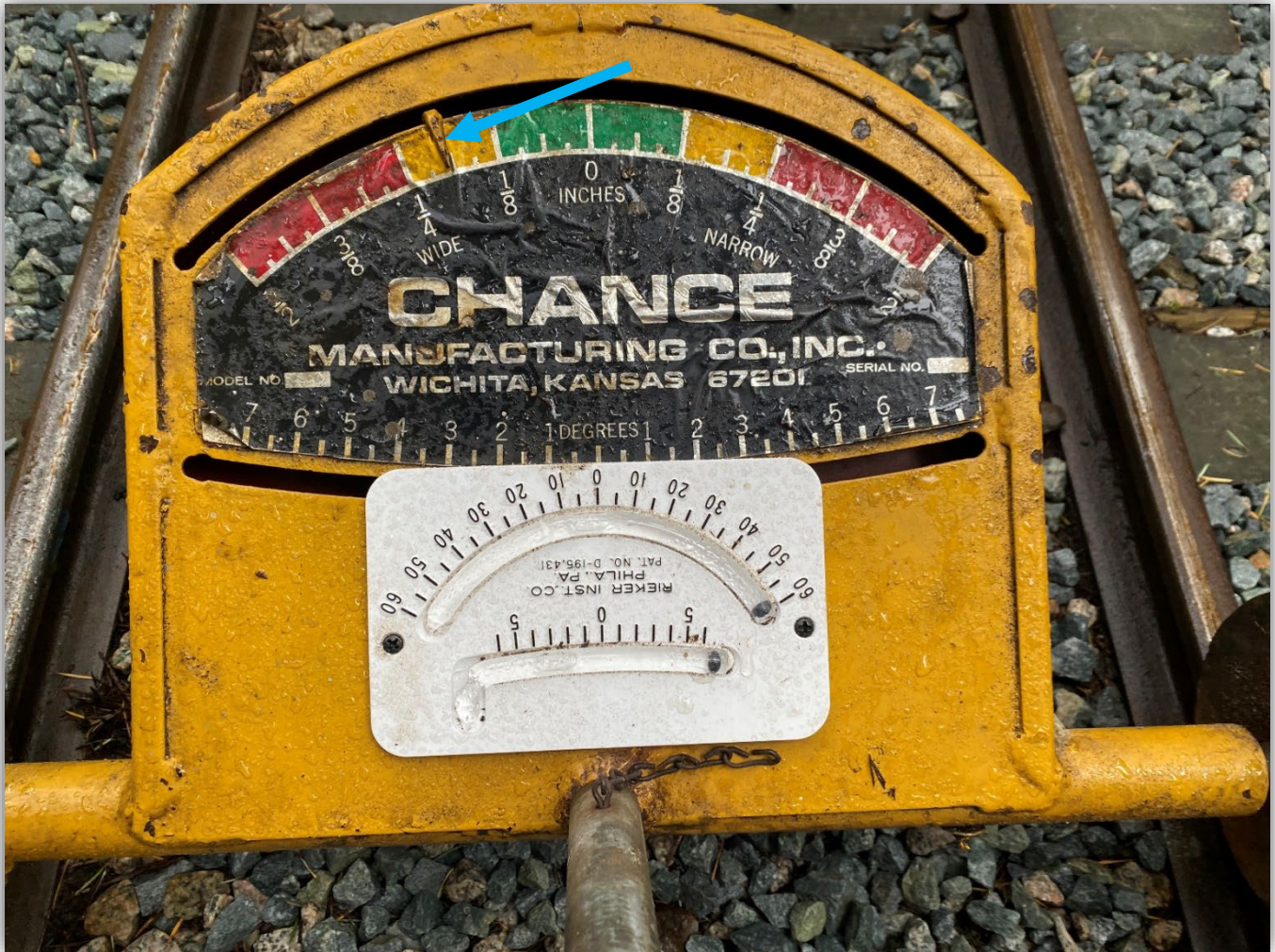
Image 7 – Track gauge with arrow showing needle indicating track width and tolerances.
