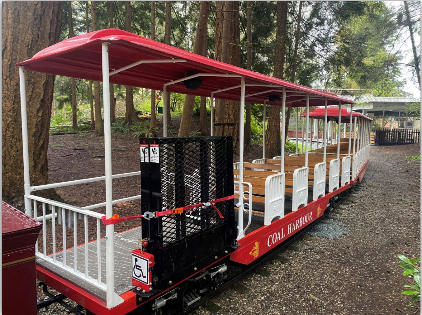
Image 2 – The accessibility car ramp folded up adding extra weight to the outside of the car.
