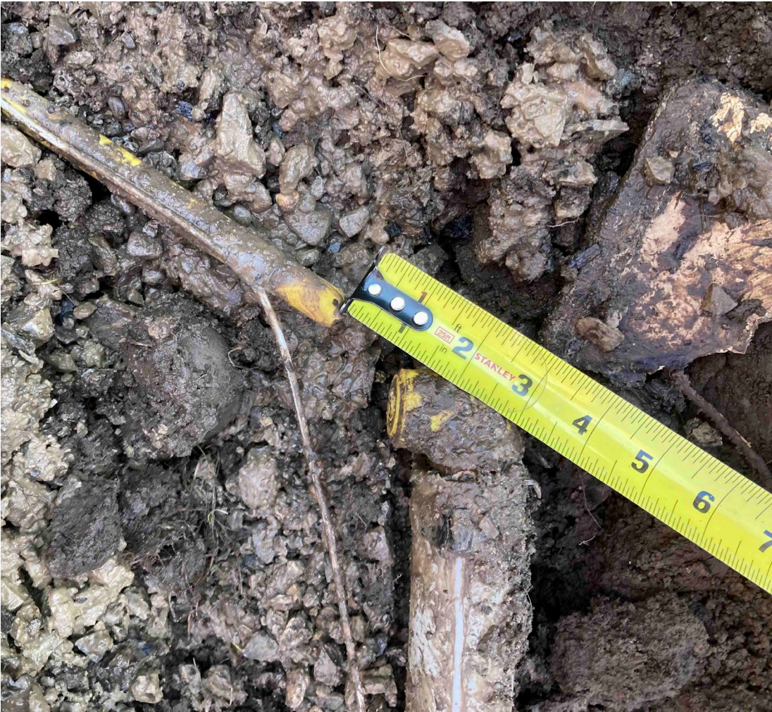
Image 7 – Close up of separated gas line that was uncovered after the incident.
