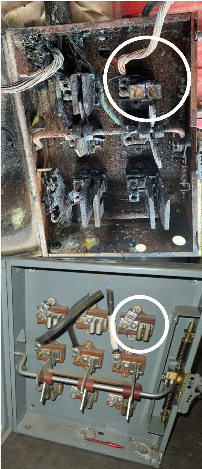
Image 4 – [Top] Damaged transfer switch bent jaw. [Bottom] Similar transfer switch normal jaw.
