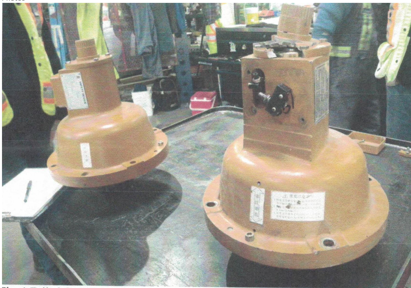
Fig. 1 Failed Over Speed Device SAJ60 on right, identical new unit on left.
