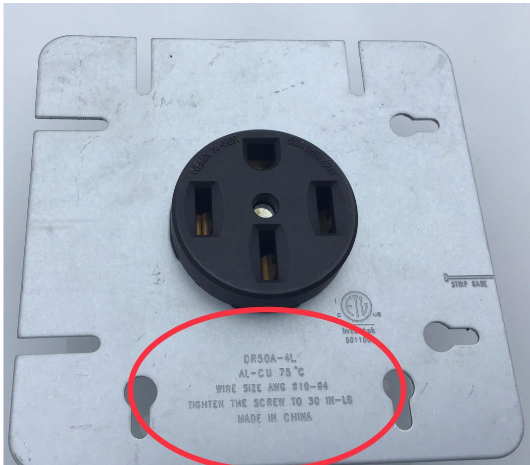
Image 3 - Manufacturer's specifications regarding; wire type, wire size and torque settings for installation.
