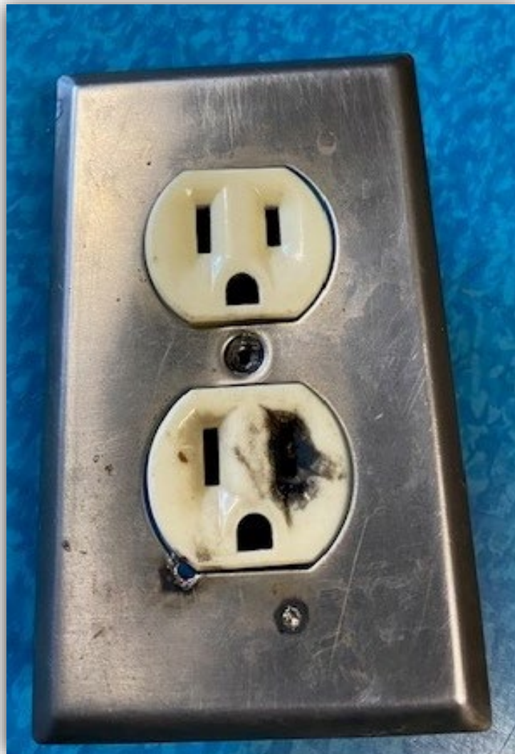
Image 1 - Original Outlet. Burned area on the receptacle and the point where the paper clip short against the metal cover plate.
