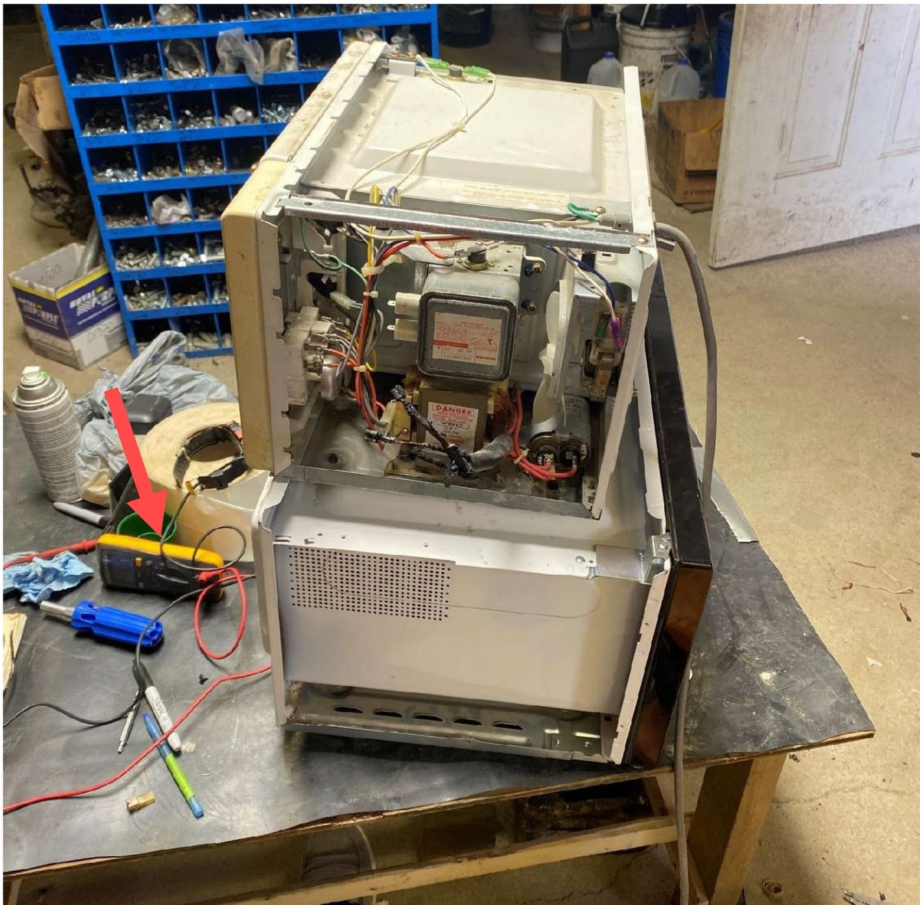
**Photo 3** – Microwave with cover removed exposing internal components. **RED** - shows digital multimeter on table next to microwave.
