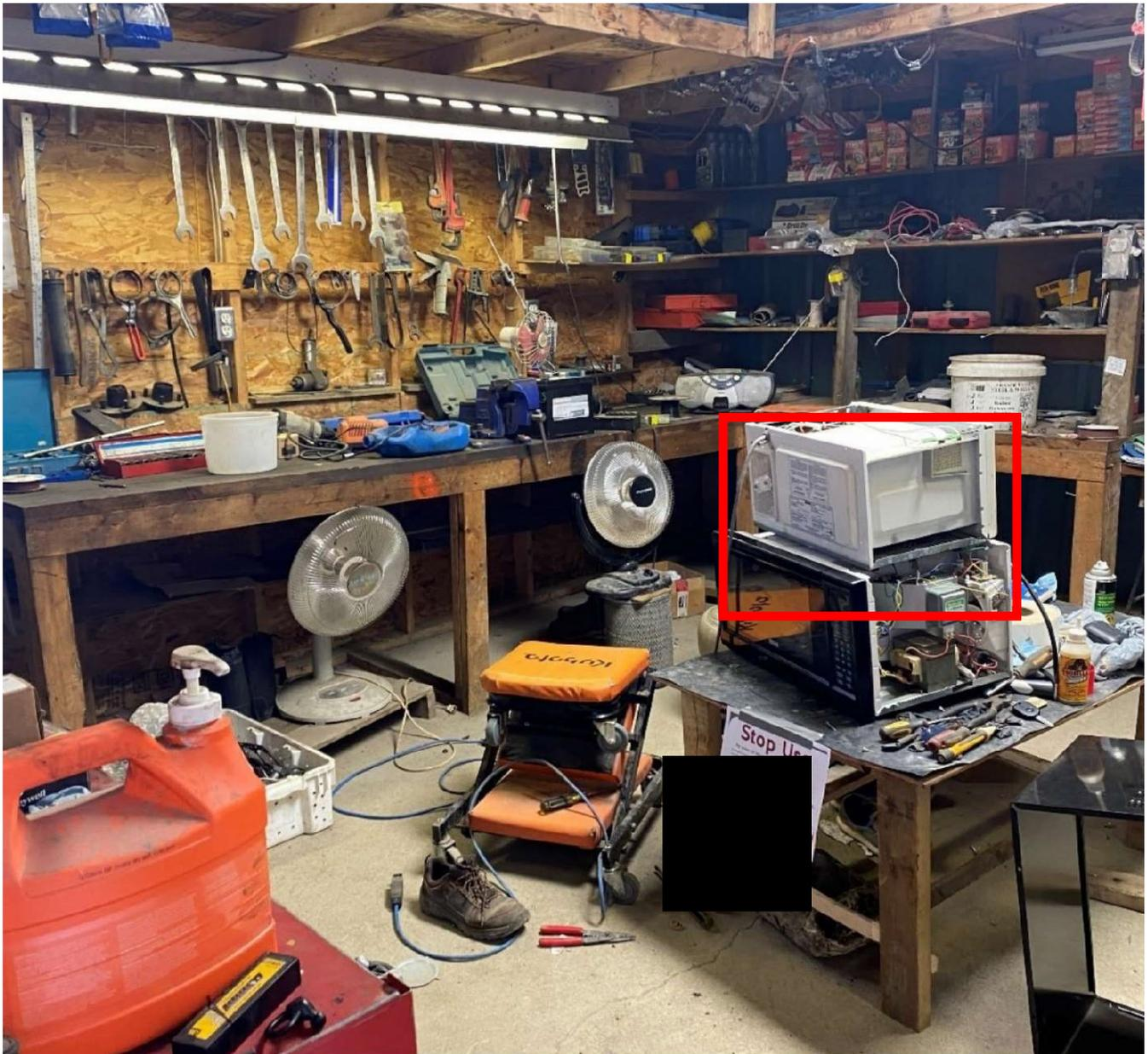
**Photo 1** – Workshop area showing two partially disassembled microwaves and tools. **RED** box showing the microwave involved in the incident. The blue extension cord on the ground was unplugged by another employee after the incident.
