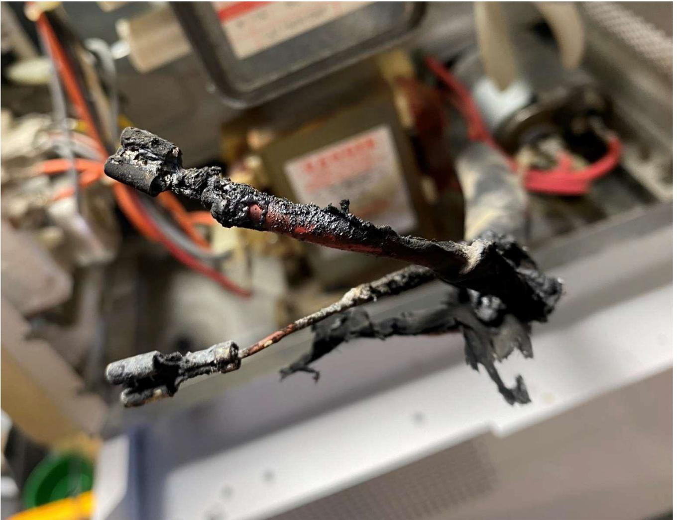
**Photo 6** – Closeup of burnt and melted high voltage wiring.
