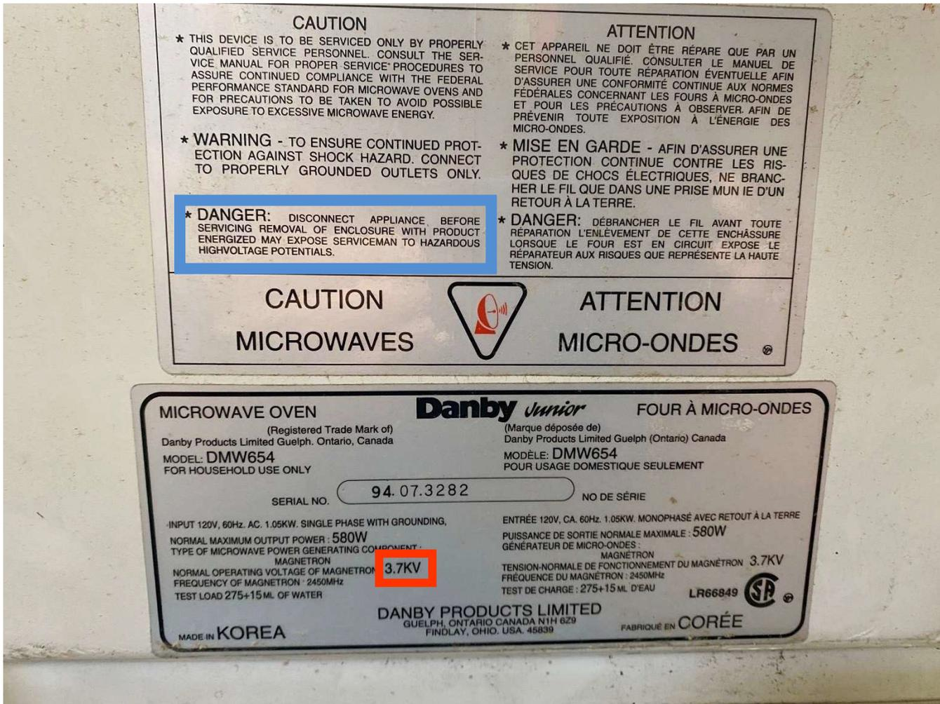
**Photo 10** – Microwave data tag with **ORANGE** box showing output voltage to magnetron at 3700 volts. Danger label in **BLUE** box identifying hazardous high voltage potentials and instructing to disconnect the appliance before servicing.
