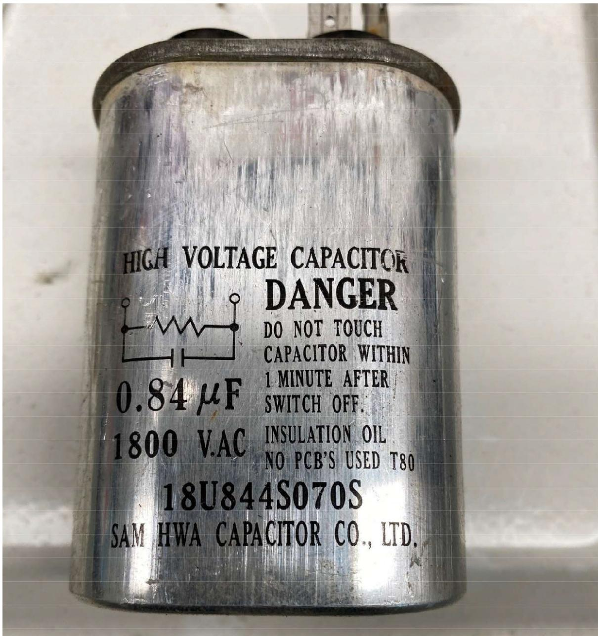
**Photo 7** – High voltage capacitor from microwave showing 1800-volt rating and danger warning.
