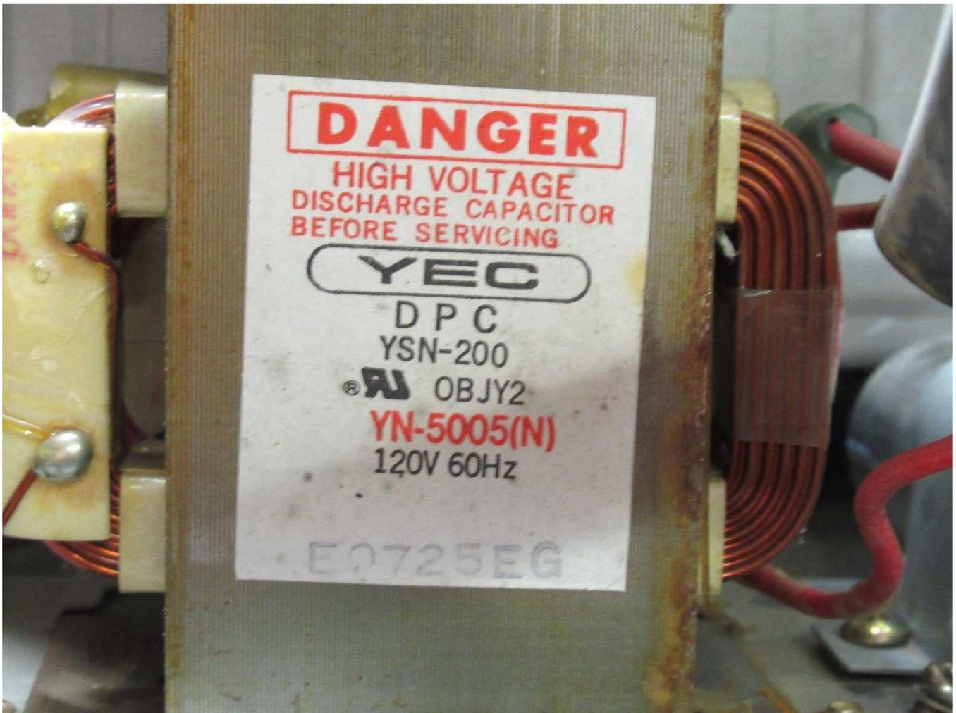
**Photo 8** – Microwave high voltage transformer with danger warning label. Voltage rating showing incoming primary voltage. Label does not state secondary high voltage output.
