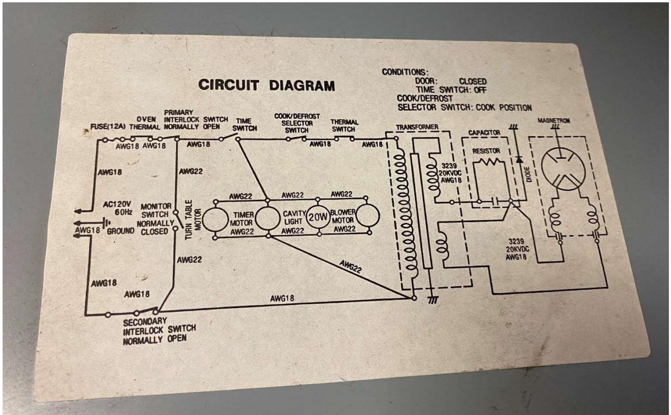
**Photo 9** – Microwave electrical circuit diagram on inside of microwave cover showing primary and high voltage circuits.
