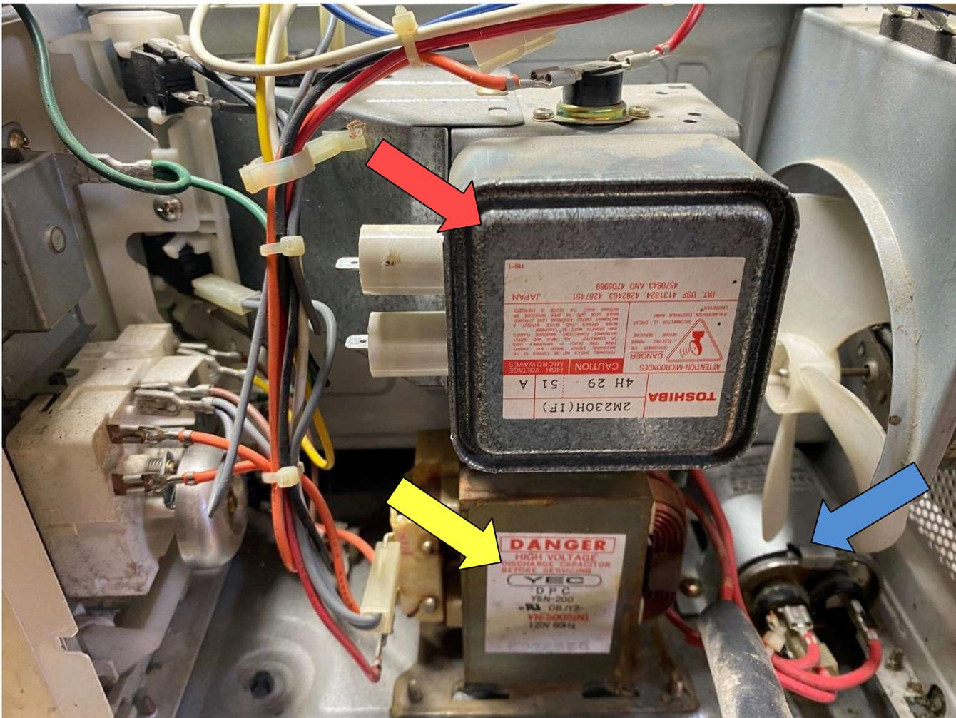
**Photo 4** – Microwave internal components: **RED** – magnetron. **YELLOW** - high voltage transformer. **BLUE** - high voltage capacitor.
