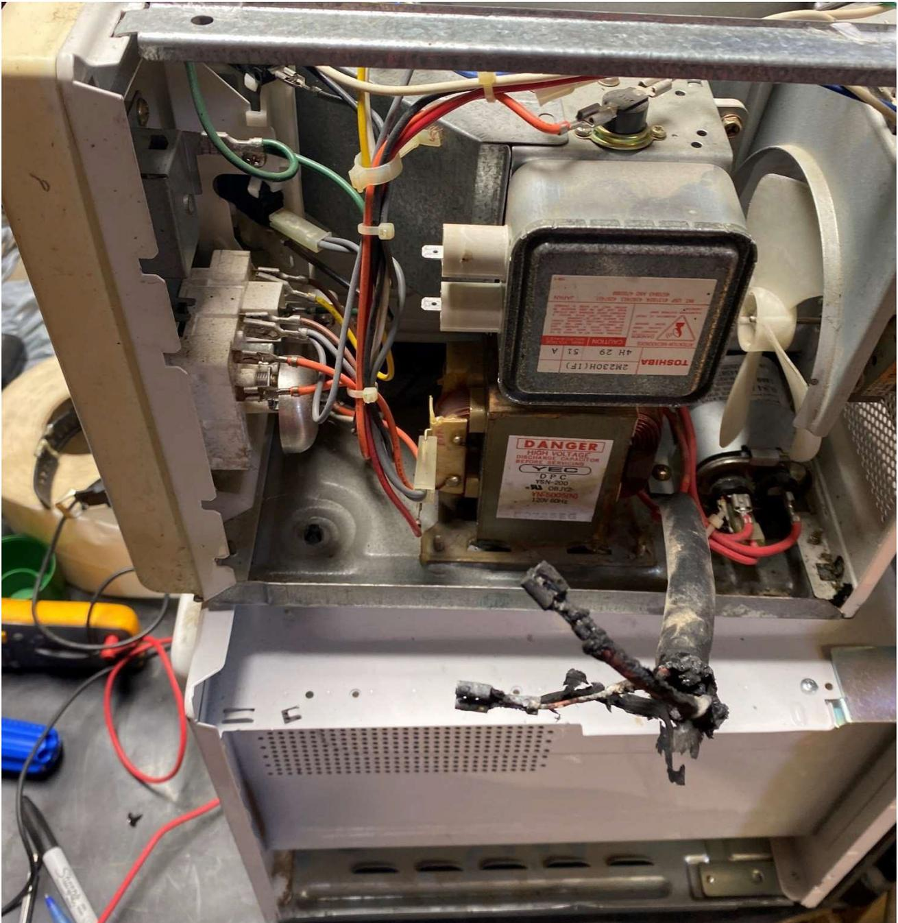
Photo 5 – Showing internal microwave components and burnt and melted magnetron wiring.
