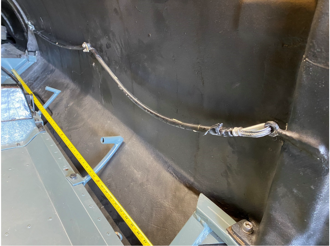
Image 4 – Cable handholds and foot pegs added to the passenger bobsleighs
