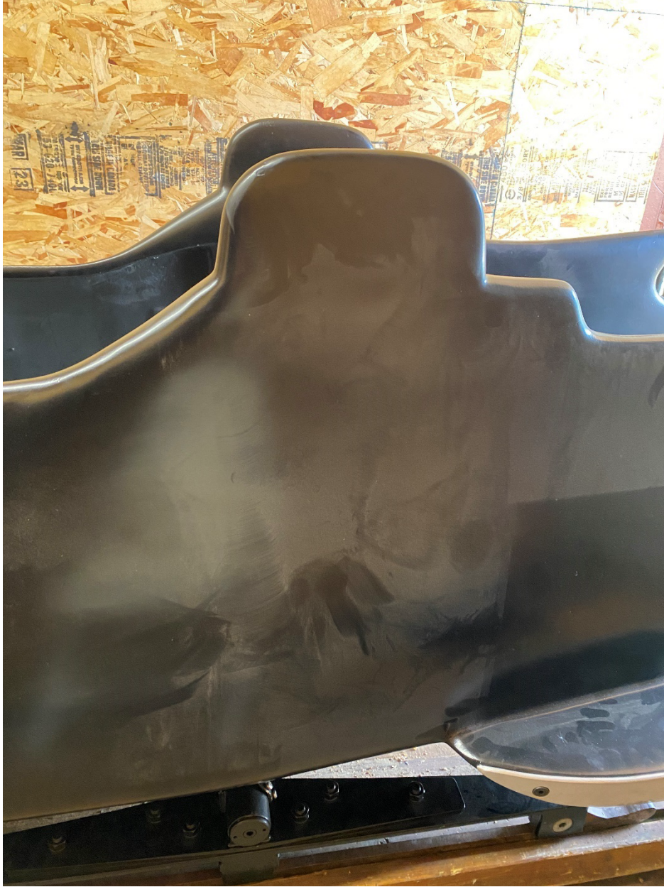
Image 3 – Modified taller sides on the public bobsleighs
