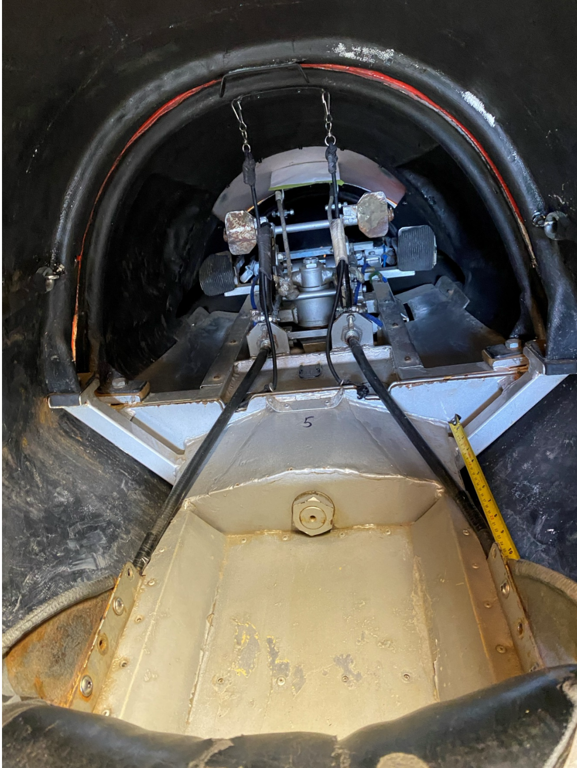
Image 5 – Front driver controls on the passenger bobsleighs
