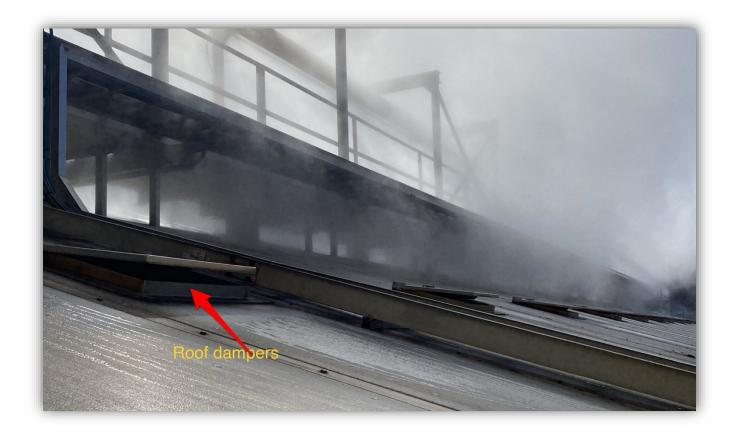
Image 2 – Red arrow showing adjustable vent dampers on the roof of the kiln.
