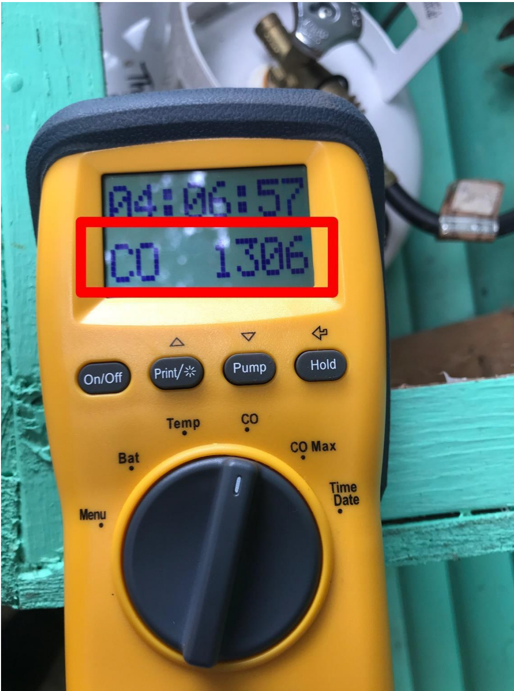
Image 12 – Carbon monoxide reading of refrigerator flue gas
