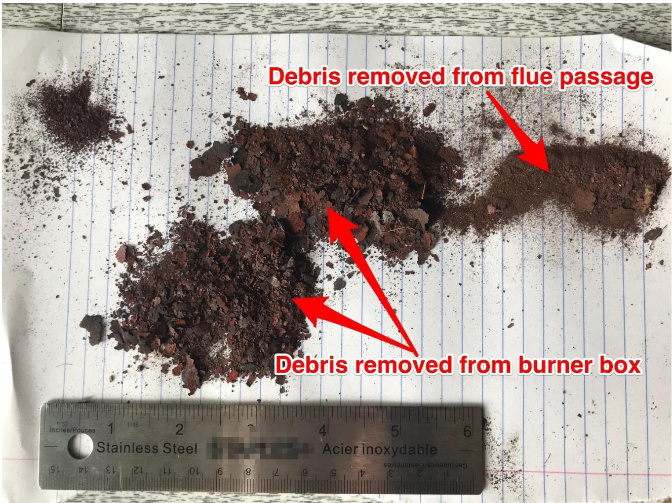
Image 15 – Corrosion scale debris removed from burner box and flue
