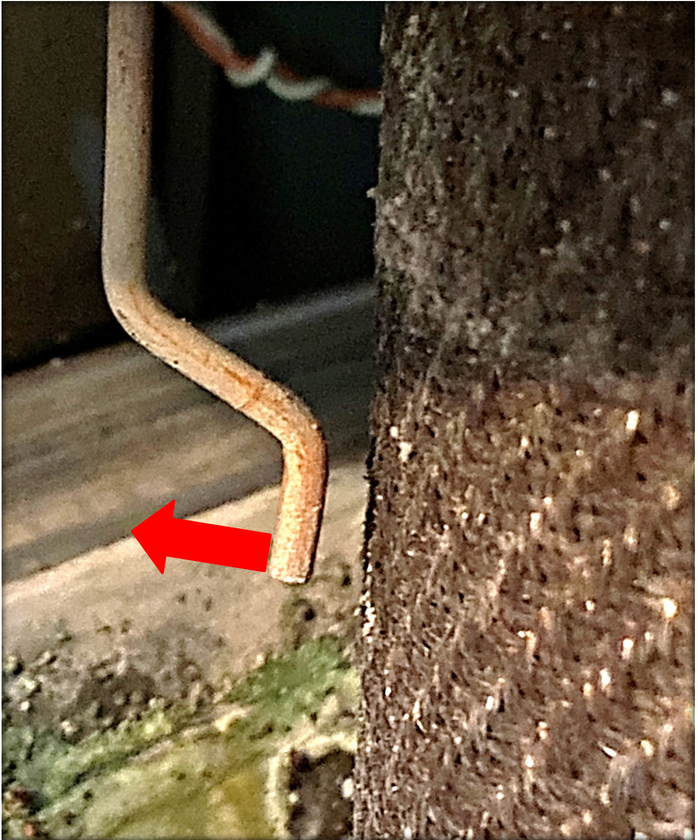
Image 5 - Single prong ignitor configuration and direction of warping away from the burner mesh due to release of stress in the metal (arrow). This warping would cause an increased arc gap.
