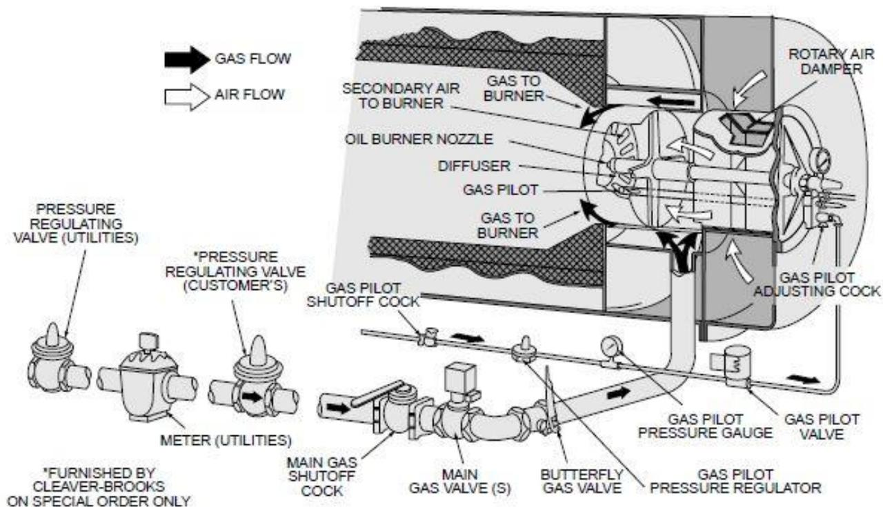
**Image 1** - From the boiler manual, showing air and gas flow paths to boiler combustion chamber. The gas flows through the burner ring gap around the diffuser to mix with the air.
