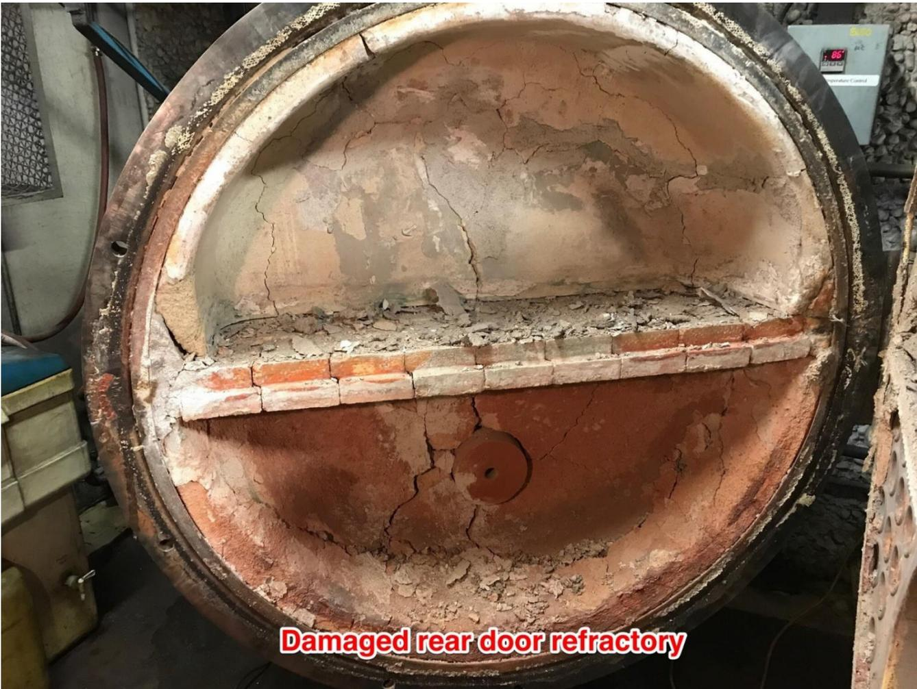
**Image 8 - Cracked and broken rear door refractory insulation**
