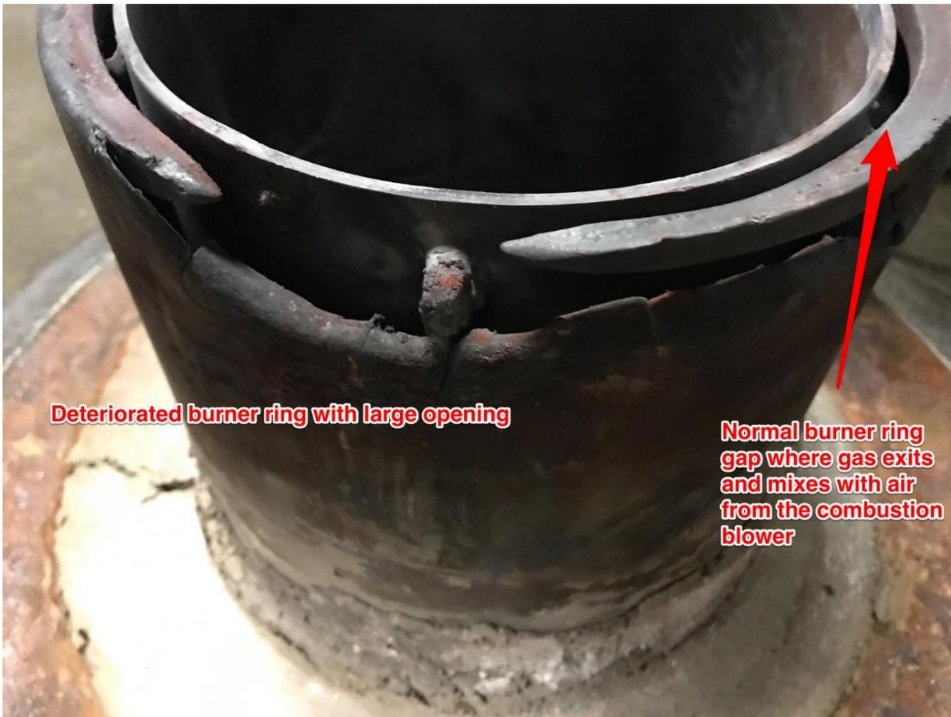
**Image 10** - Burner housing with deteriorated ring and large gas port opening. The air diffuser gets positioned in the middle circular area of the burner housing.
