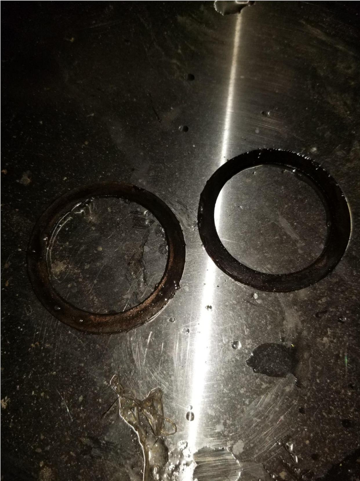
Photo 4 (Submitted by client) Failed ammonia strainer gaskets
