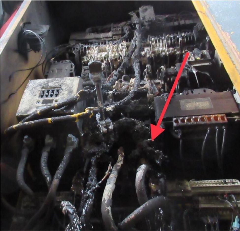
This photo is of the inside of the control panel located inside the operators cab after the incident. The red arrow indicates the location where the operator touched right before the unintended release of electrical energy occurred and resulting fire. The location appears to be on the line side of the control panel disconnect.
