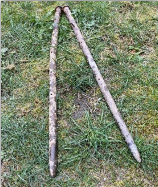
Image 4 – Metal stakes used for concrete forming braces and the length of metal stakes.
