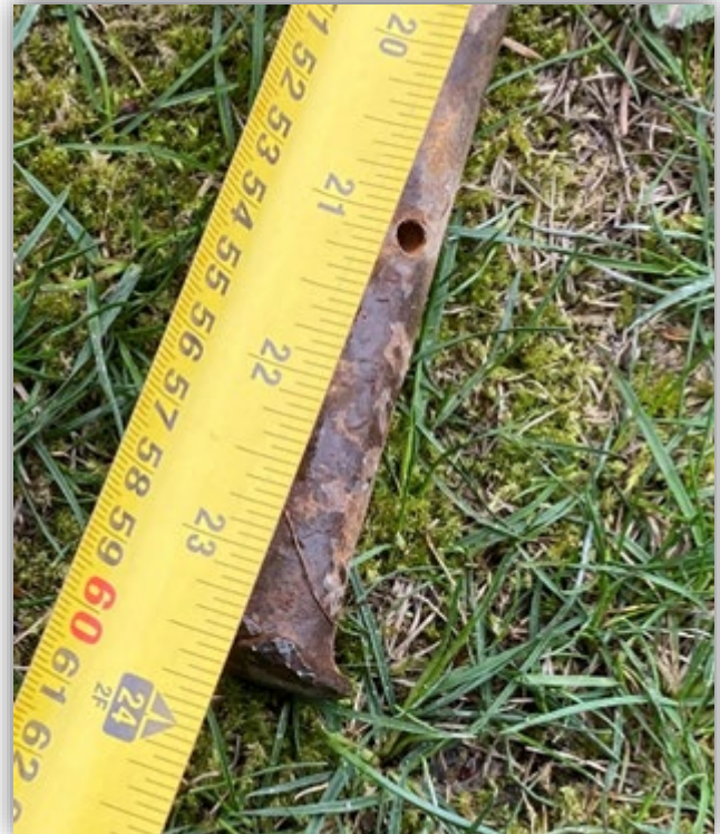
Image 4 – Metal stakes used for concrete forming braces and the length of metal stakes.
