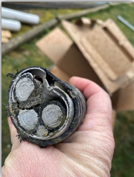
Image 3 – Damaged cable from the concrete forming stake.
