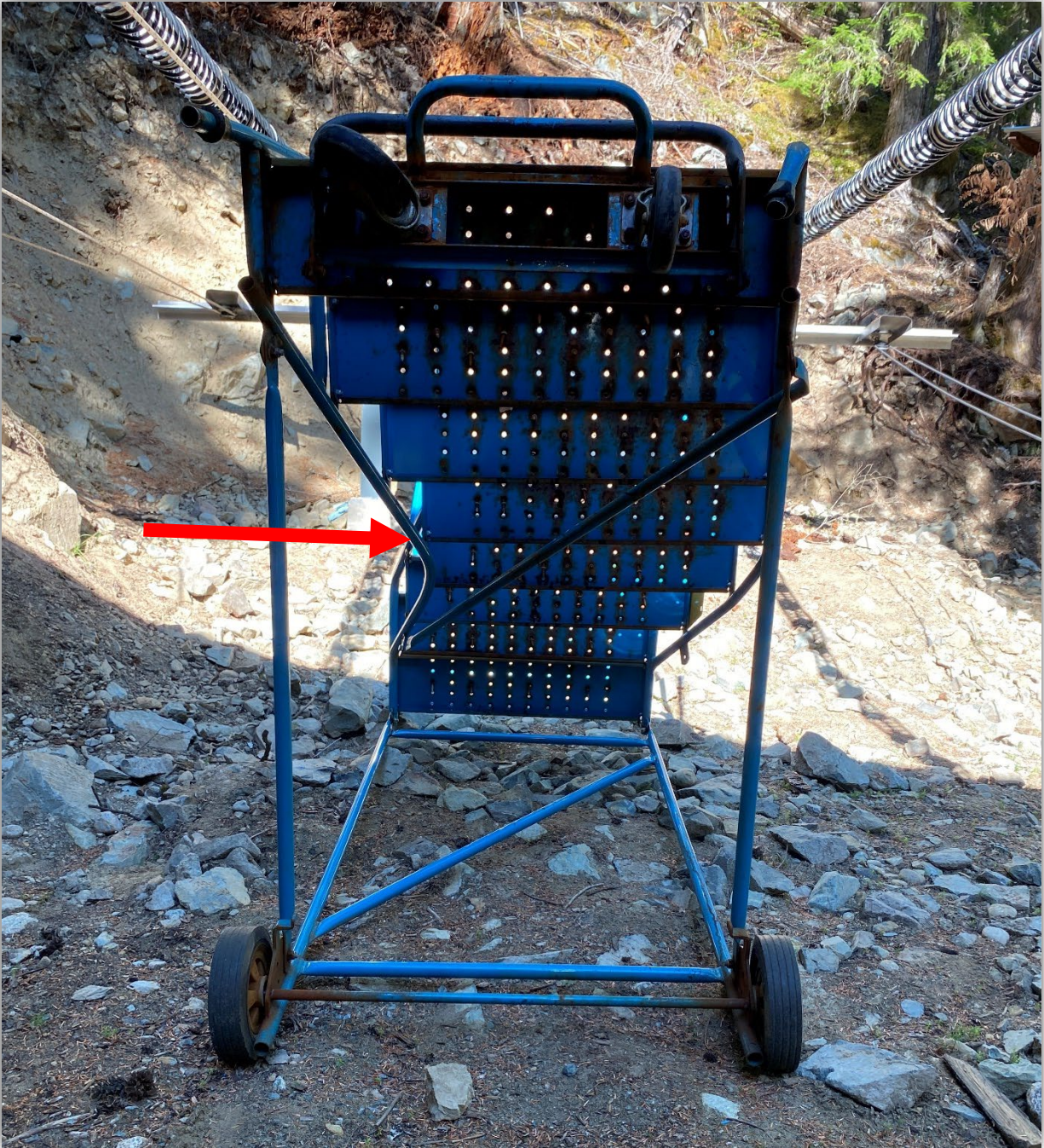
Image 11 – Damaged staircase bent by the impact from the rider.
