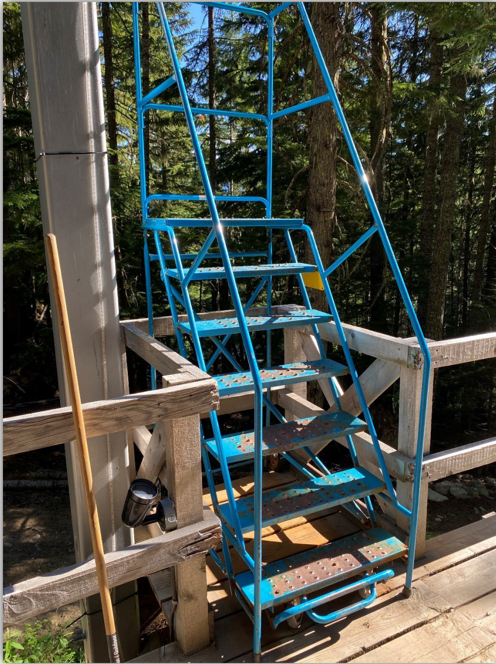
Image 6 – Rolling staircase placed in the stowed storage location out of the path of the riders.
