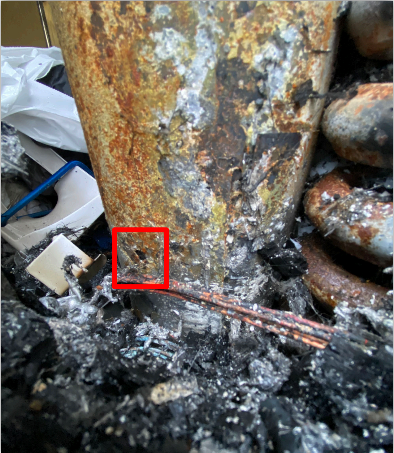
Image 5 - Hole in the combustion chamber where wire contacted the combustion chamber. Hole was found located directly at the base of the burn pattern.
