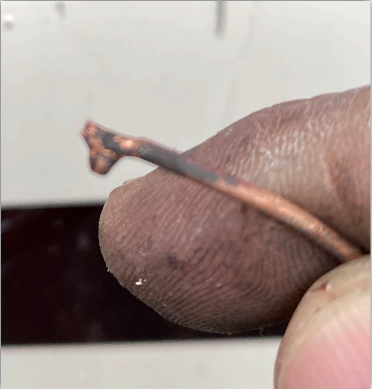
Image 6 - Area on wire that it is believed to have come in contact with combustion chamber. Note deformation from heat caused by arcing.
