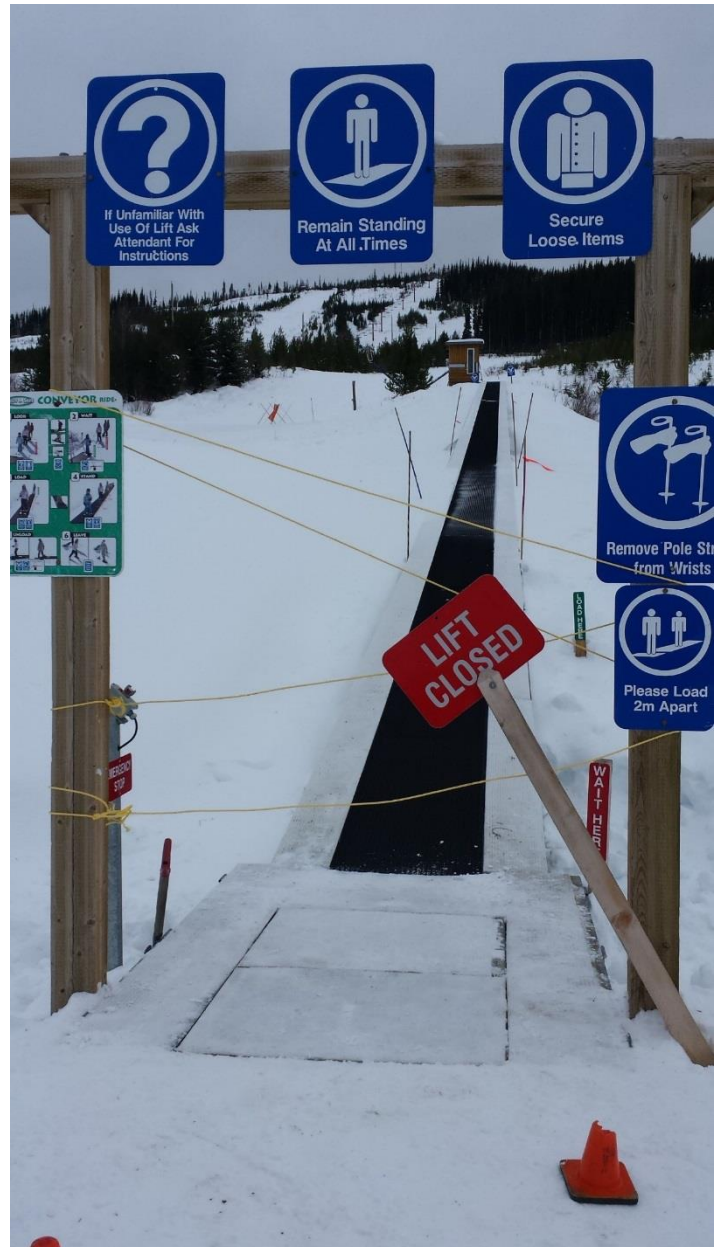
Figure 3: Photograph of the conveyor tail unit with the centre cover plates.
