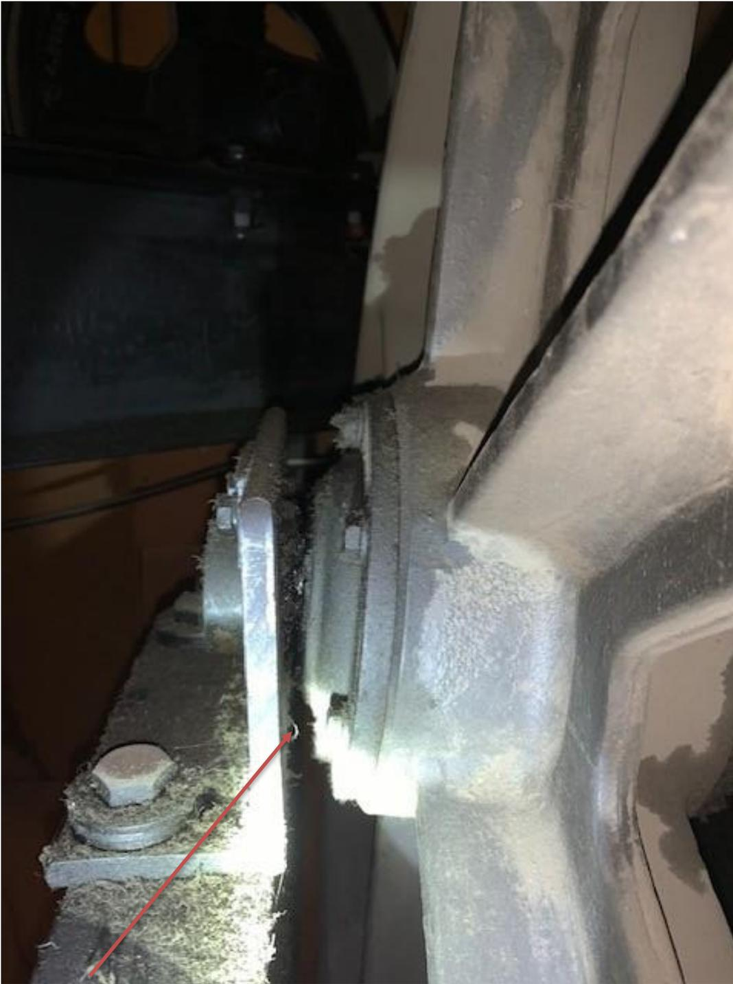
**Photo 2** - Photo shows the sheave out of plumb and tilted towards one of its sides.
