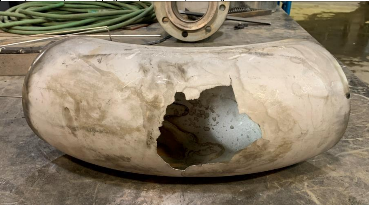
Failed 316 SS Sch 10 6" Elbow
