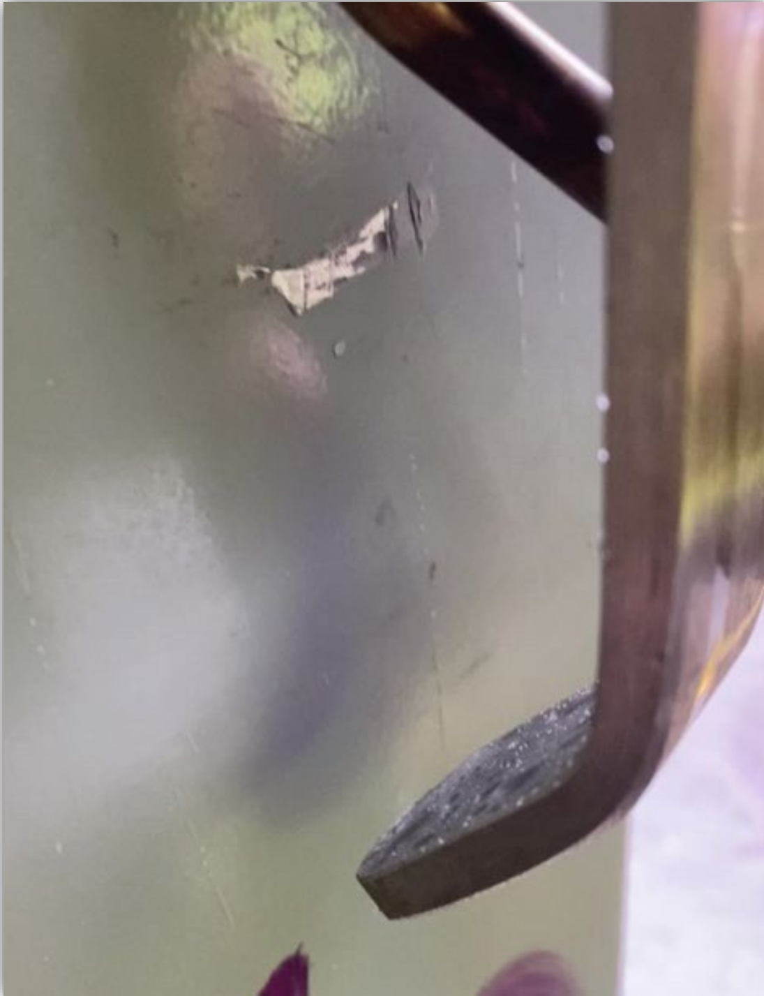
Image 7 – Scrape marks caused by tools during tampering and padlock removal by unknown persons prior to incident.
