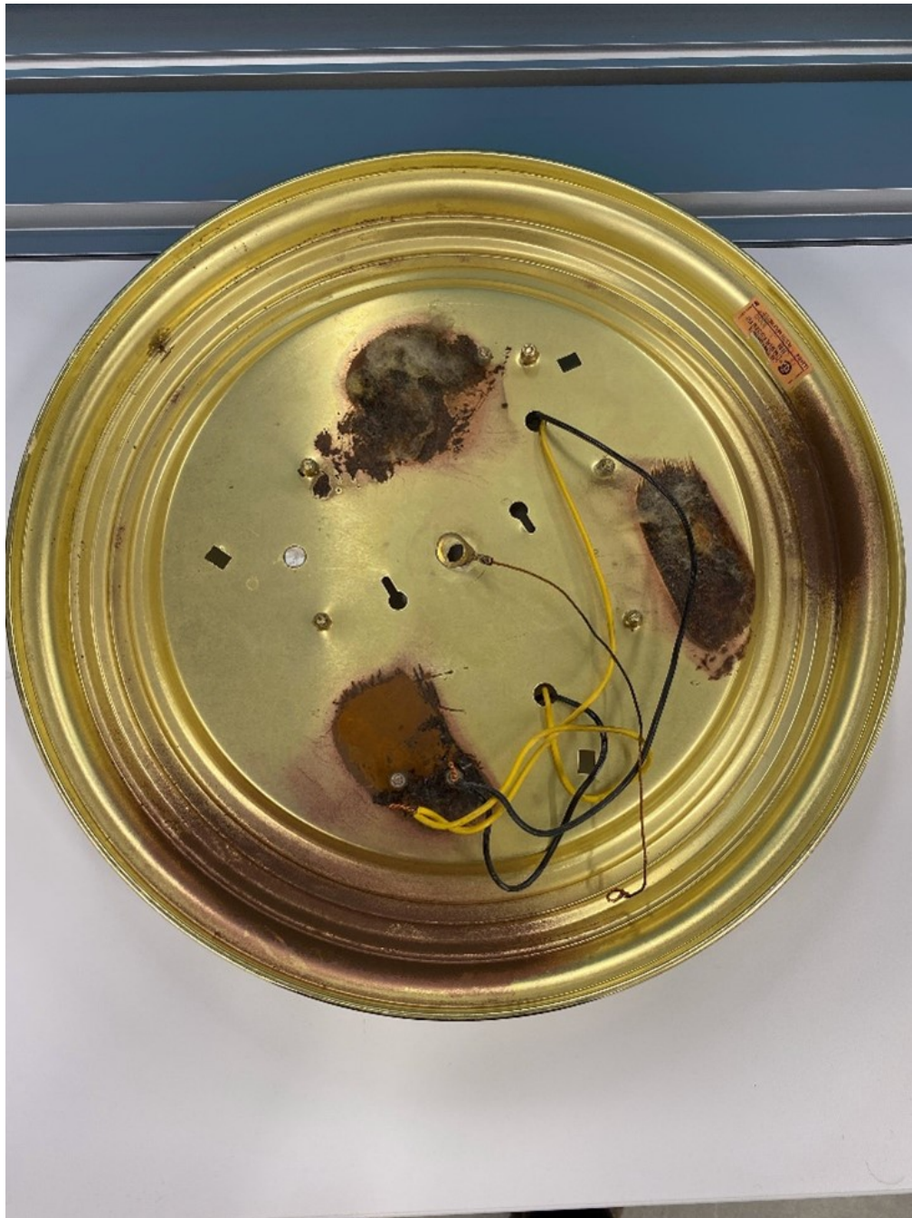
Image 2– Back side of fixture showing discolouration and remnants of insulation barrier that was once in place.
