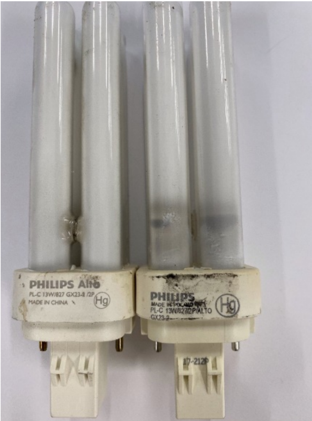
Image 5 – 13W fluorescent lamps as approved for the fixture.
