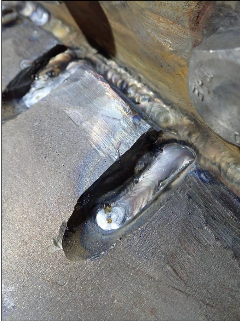
Figure A-6 Typical crack after hot pass is placed.
