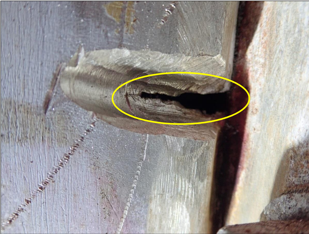
Figure 7: Close up view of typical weld crack size at the inner shell surface. (Source: Acuren report).
