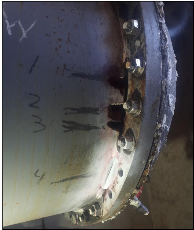
Figure 5: Location of 10 weld cracks found by ultrasonic testing. (Source: Acuren report)
