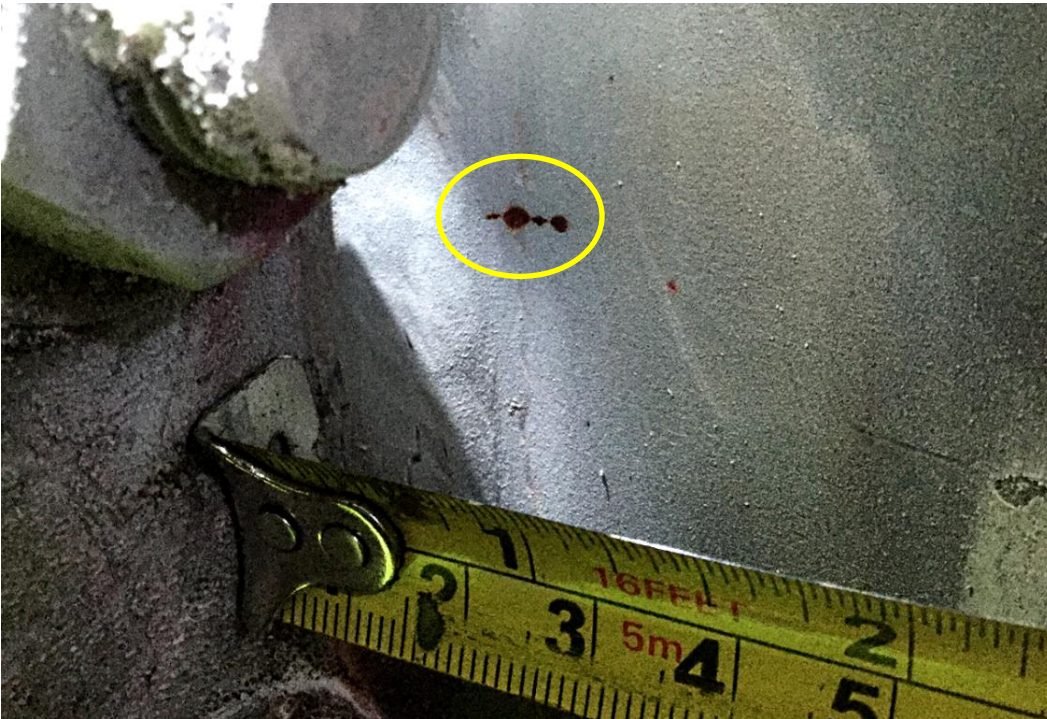
Figure 3: First crack found in the weld, revealed using liquid dye penetrant inspection. The crack was 0.250-inches-long and extended from the weld into the parent material.
