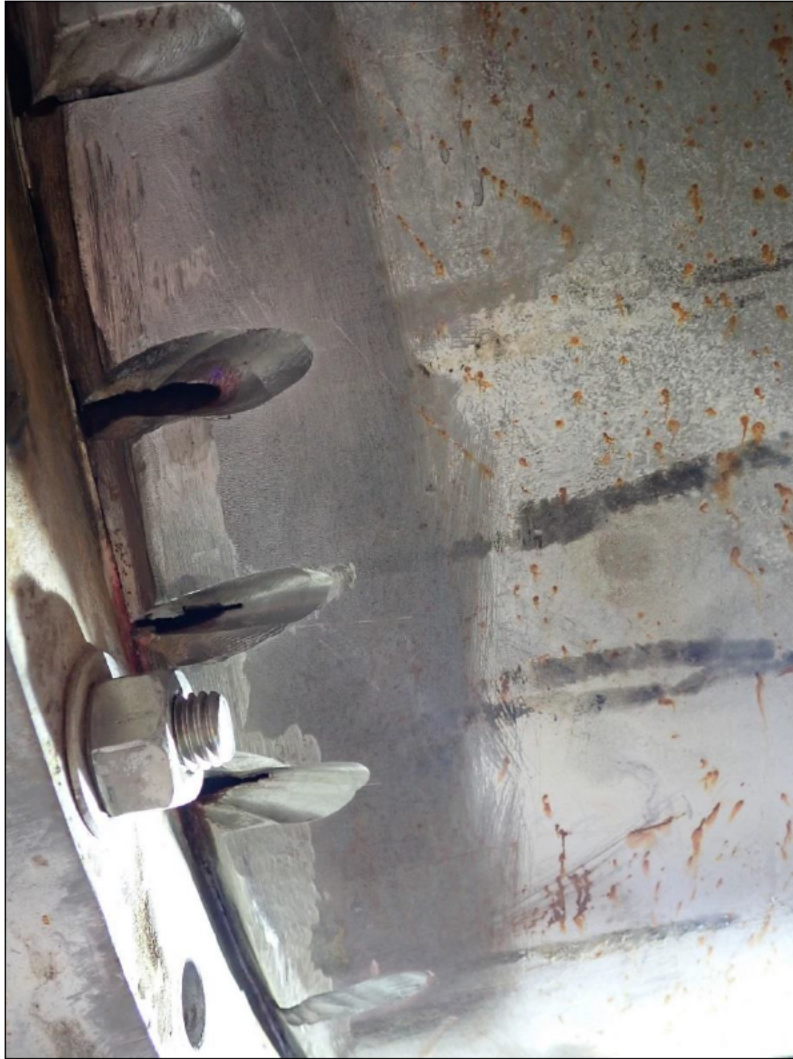
Figure A-3 Short axial crack entering the shell of the vessel.
