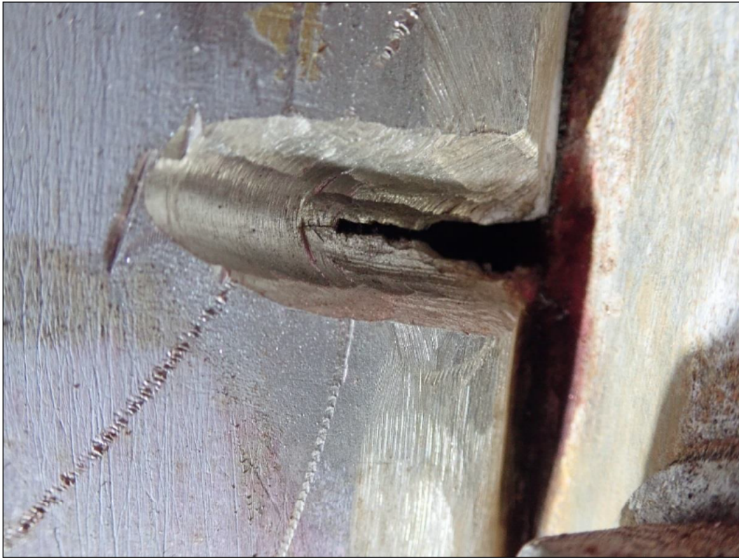
Figure A-4 Ground out crack showing opening of 1 -2 mm and depth of 3/8”.
