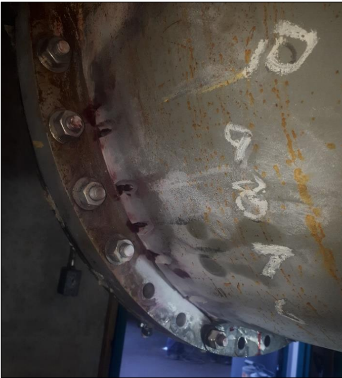
Figure 5: Location of 10 weld cracks found by ultrasonic testing. (Source: Acuren report)
