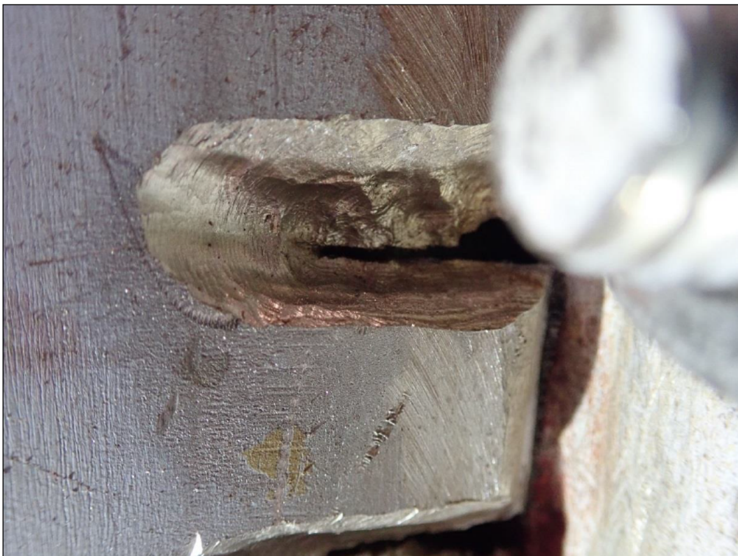
Figure A-5 Second ground out crack showing opening of 1 -2 mm and depth of 3/8”
