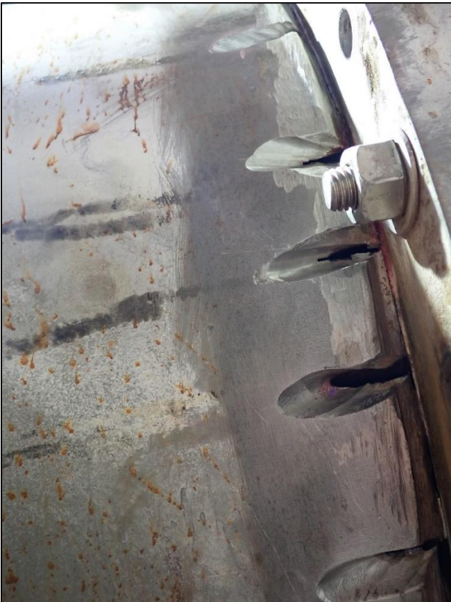
Figure 6: Large internal cracks found when welds ground to reveal inner shell surface. (Source: Acuren report)
