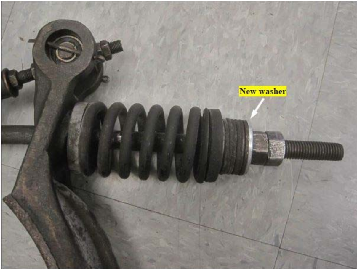
Figure 4 Shows the addition of Flat washers for tension adjustment. Photo courtesy of Acuren Group Inc.
