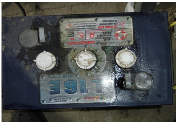
Incorrect bolt sizes used for battery connections, causing lead post to melt, burning a hole in the cell:
