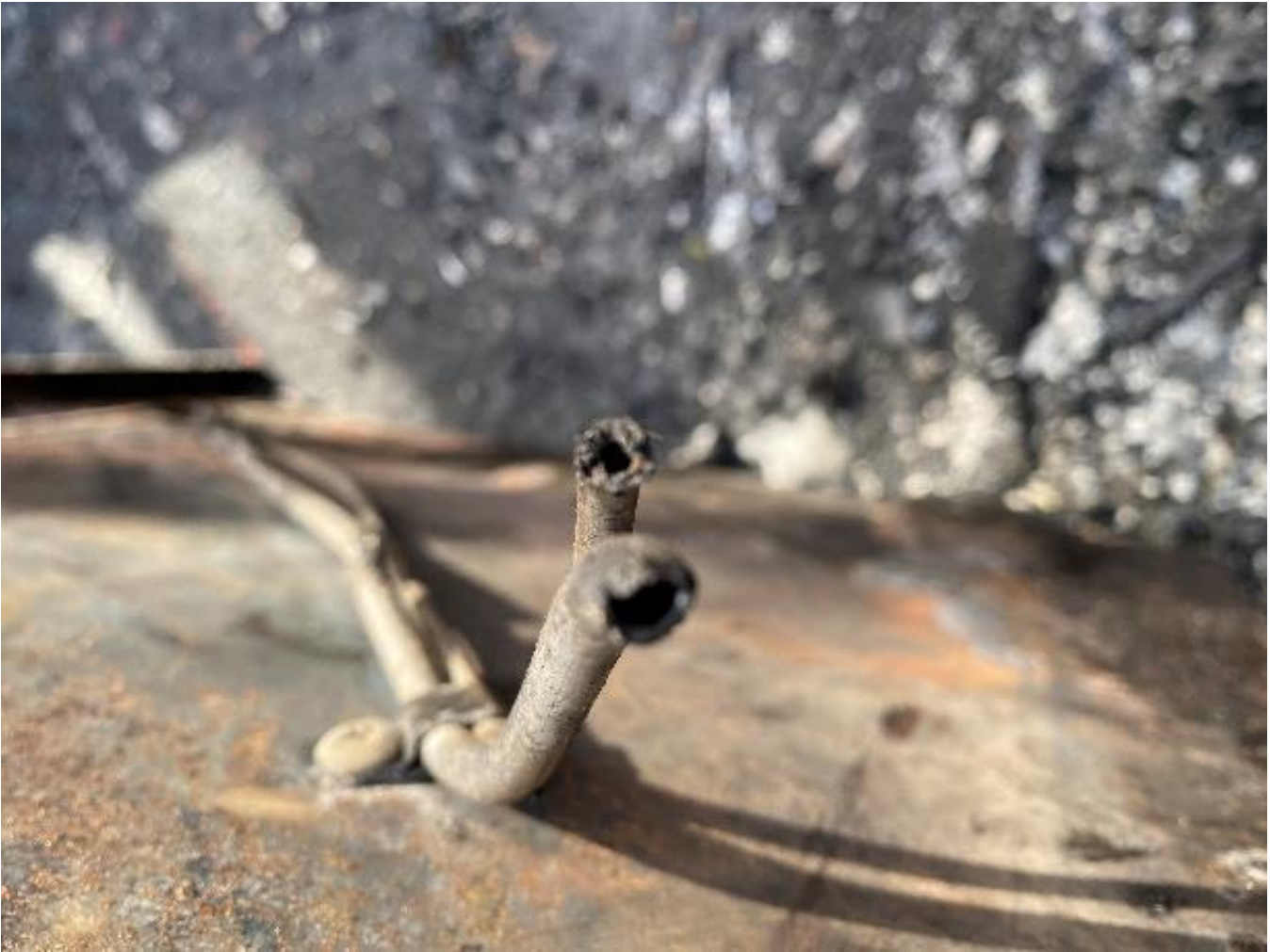
Image 2 - Corroded oven gas tubing behind stove
