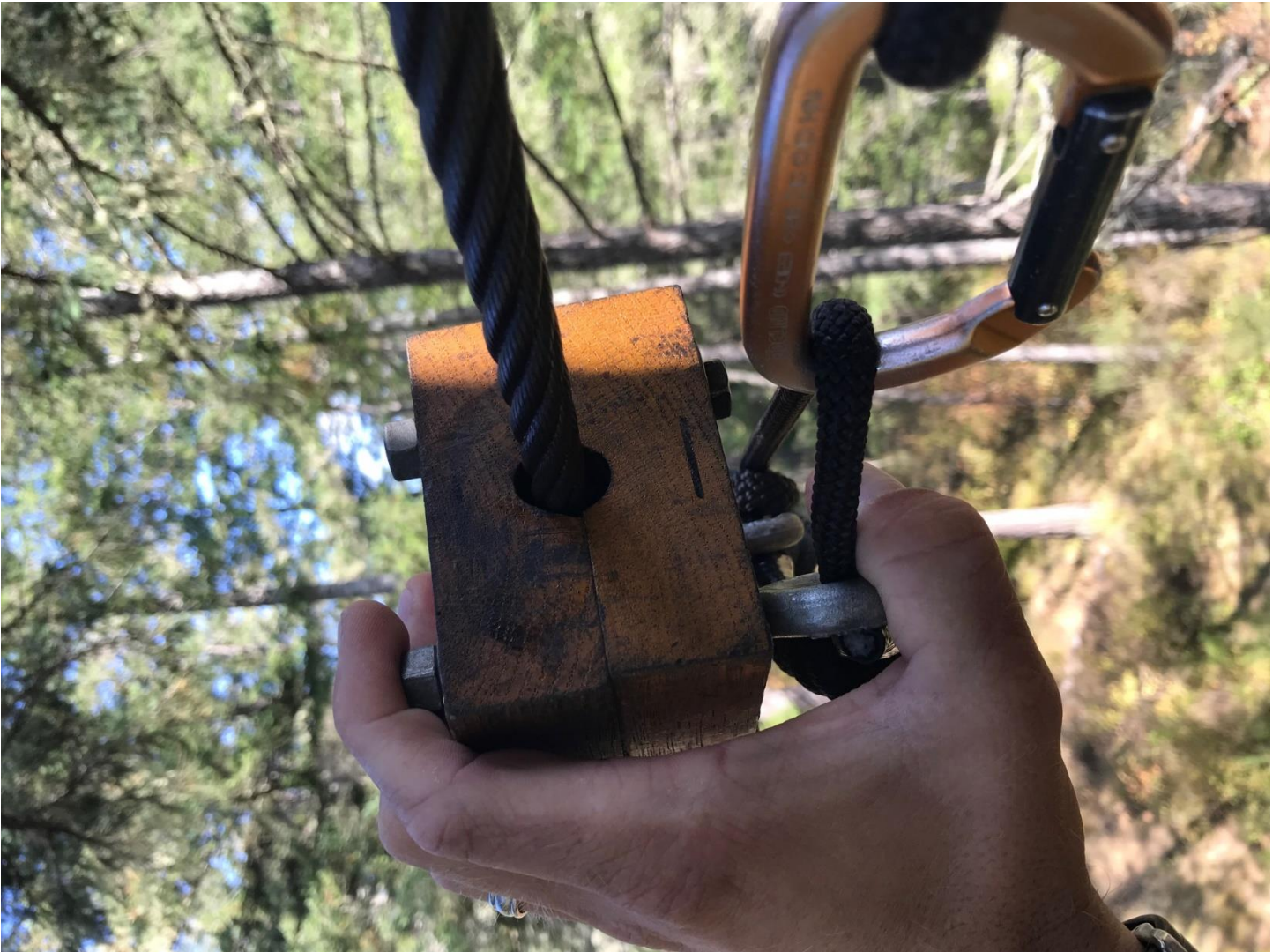
Back side of brake block where rope from pulley setup attaches
